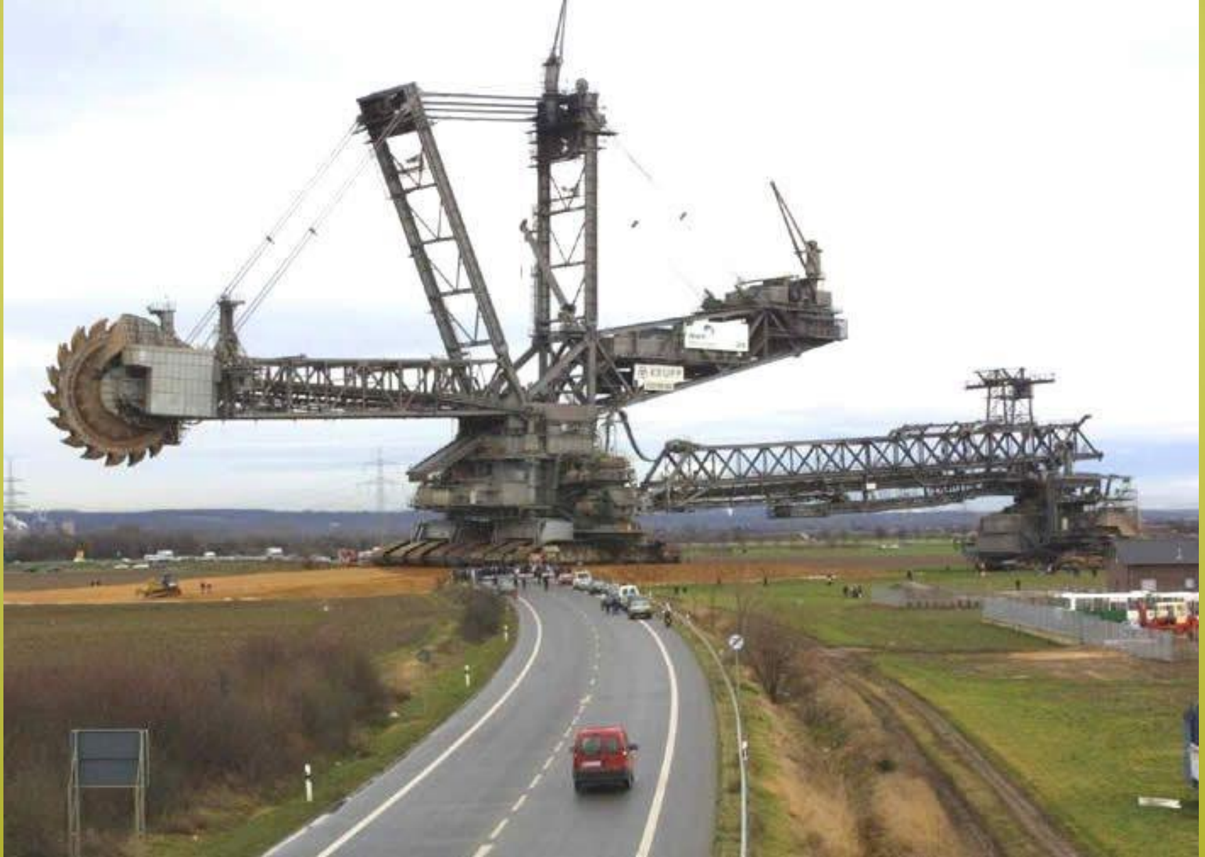
Large bucket wheel extractor being moved through Germany. Moves 10 meters per minute. Takes 5 people to operate. Used in strip mining
