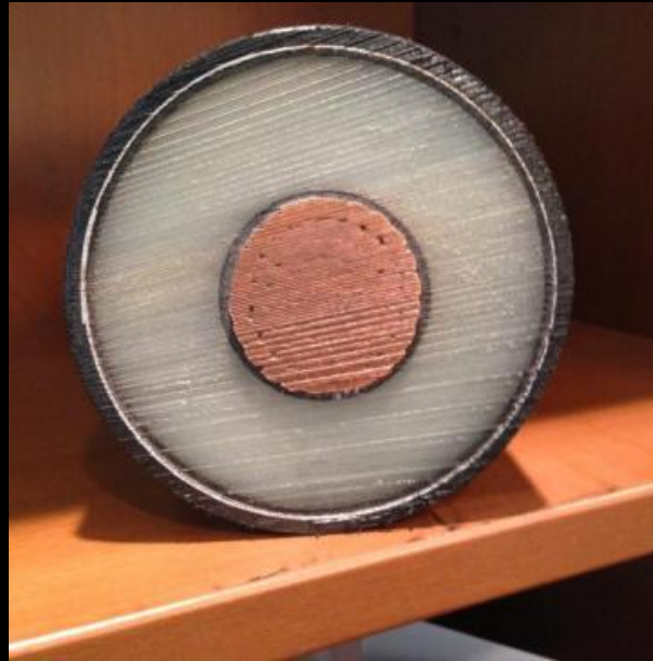
Large gauge insulated copper cable with 230,000 volt capacity. A single strand in the cable is much larger than all seven strands in the household wire.
