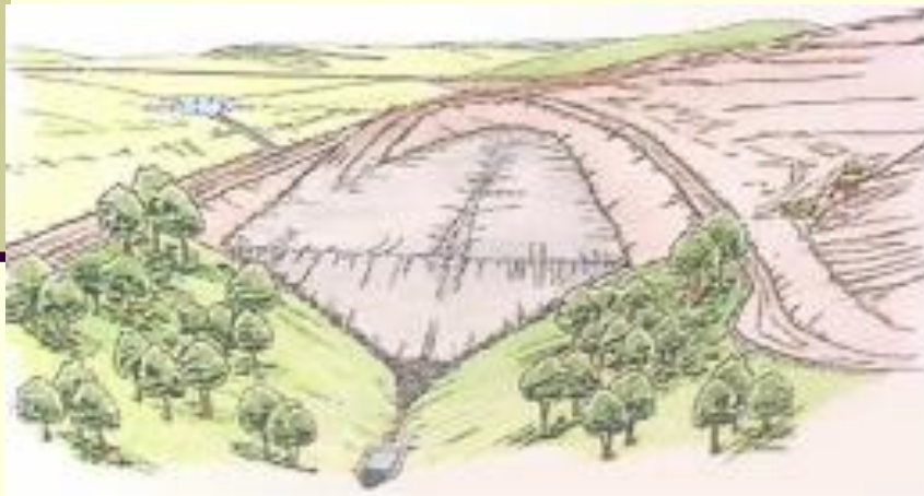
(3) Completed Fill Placement
