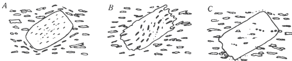
Fig. 15-2. A. Inclusion of a fine early schistose fabric, indicating the porphyroblast grew before coarser grains of the groundmass. B. Included sigmoidal fabric indicating porphyroblast grew during gradual rotation, presumably due to simple shear within the groundmass. C. Partially replaced relicts parallel to groundmass fabric, indicating post-tectonic growth of the porphyroblast.
