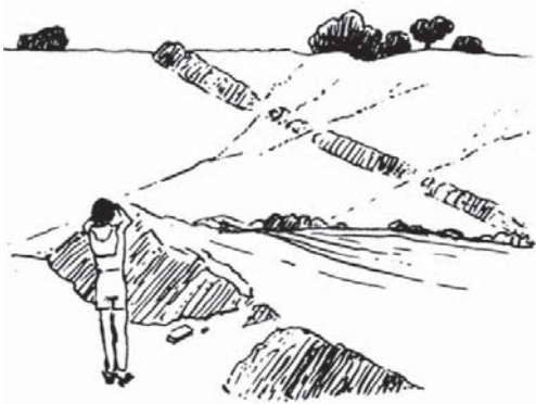
Fig. 3-6. Sighting a strike line across a valley. The dip is taken from the same position and averaged over the entire outcrop on the far hillslope.
