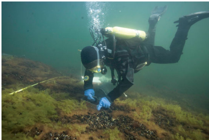
Plate 9.2 Placement of frames along a transect line perpendicular to the depth curves. Observations are made within each frame only. Frames are either placed at fixed depth intervals or distance from shore.
