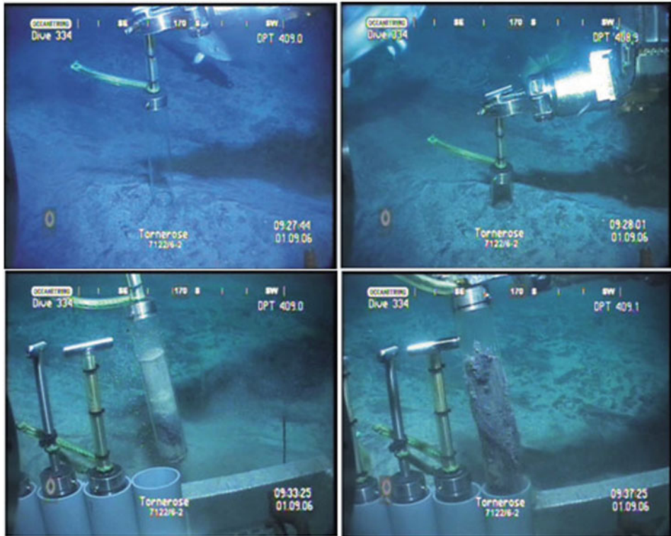
Fig. 7.9 Remotely Operated Vehicle (ROV) push cores in use in the Barents Sea. (Images © SERPENT.) (For a colour version of this figure, see Plate 7.5.)
