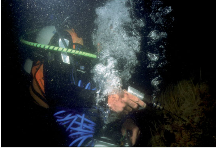
Plate 4.8 A diver-operated air drill being used to mark a sub-littoral monitoring station in Milford Haven. © Colin Munro.
