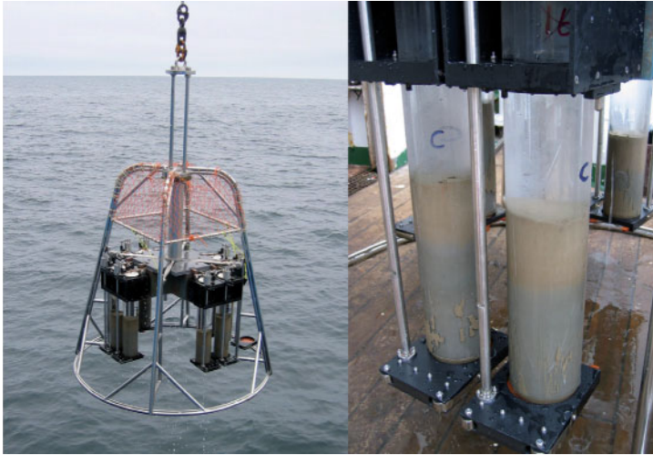
Plate 7.4 The Bowers and Connolly Maxicore being deployed and a close-up of two successful cores from the deep sea. (Images © the University of Aberdeen, UK.)
