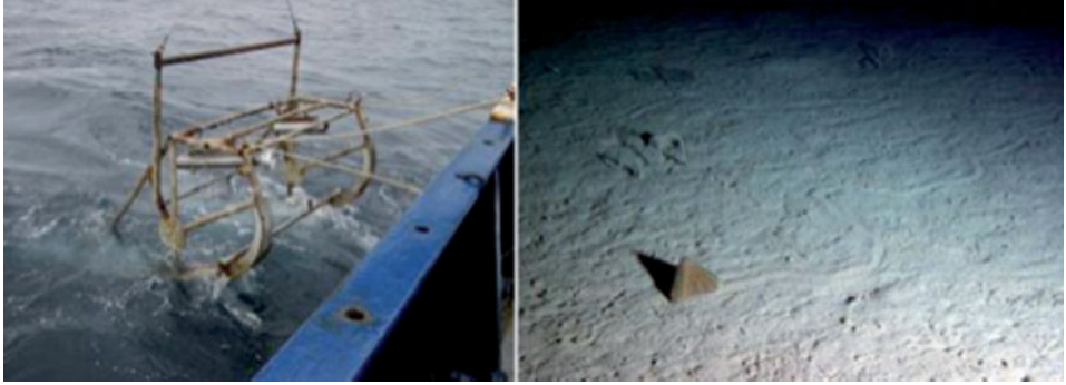
Plate 7.6 An example of a towed camera sledge; the Scripps camera sledge (left) and an image from the deep-sea floor (right). (Images © Ken L. Smith Jr., MBARI, USA.)
