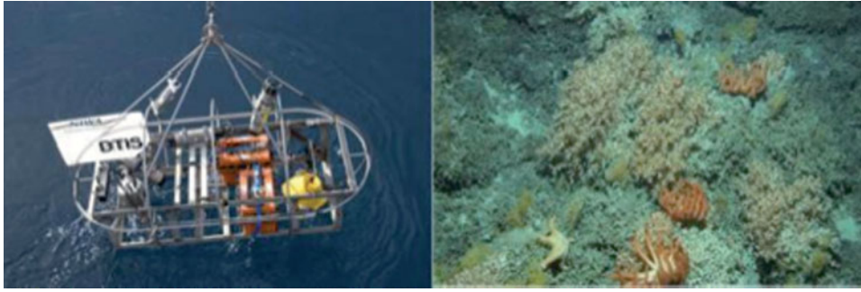
Fig. 7.11 The Deep Tow Imaging System (DTIS) (left); an example of an image taken of fragile coral mounds taken by DTIS (right). (Images © the National Institute of Water and Atmospheric Research, New Zealand.) (For a colour version of this figure, see Plate 7.7.)
