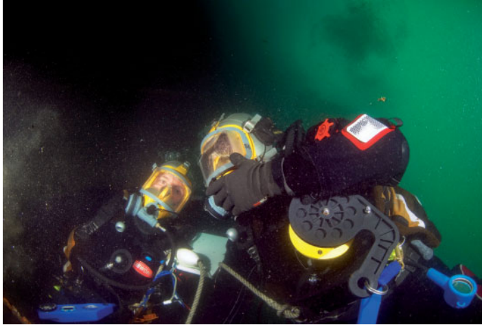
Plate 4.2 Plymouth University Diving & Marine Centre professional diving students using positive pressure full-face masks. Diver on right can be seen operating press-to-talk through-water Buddy Phone voice communications. © Colin Munro.
