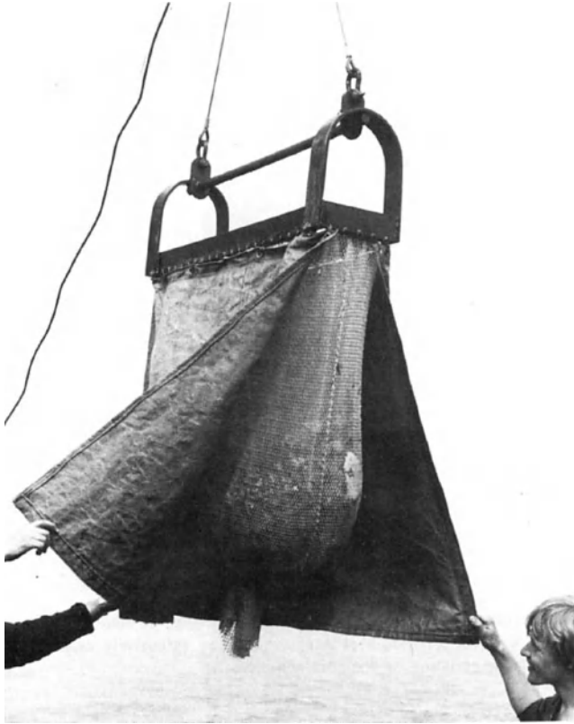
Fig. 5.5 Dredge with runners as used by the Marine Laboratory at Plymouth. The width is 1 m and the net is protected by canvas strips on either side of the net.
