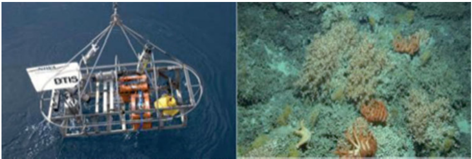
Plate 7.7 The Deep Tow Imaging System (DTIS) (left); an example of an image taken of fragile coral mounds taken by DTIS (right). (Images © the National Institute of Water and Atmospheric Research, New Zealand.)
