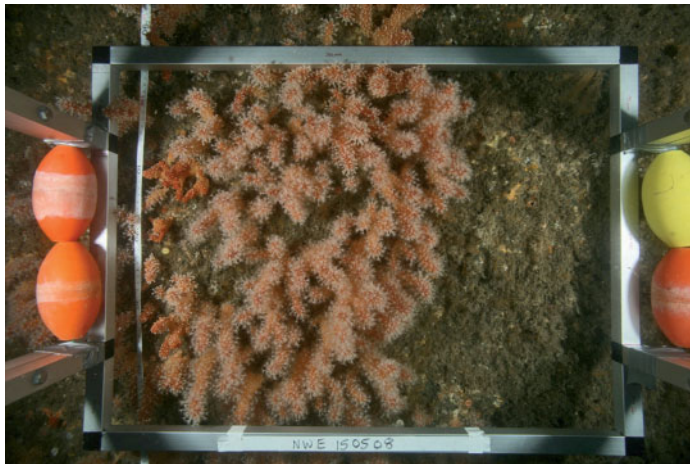
Fig. 4.5 A photo-monitoring framer being used to photograph Alcyonium glomeratum soft coral colonies. Orange floats are to compensate for weight of the framer. © Skomer Marine Nature Reserve, Countryside Council for Wales. (For a colour version of this figure, see Plate 4.3.)
