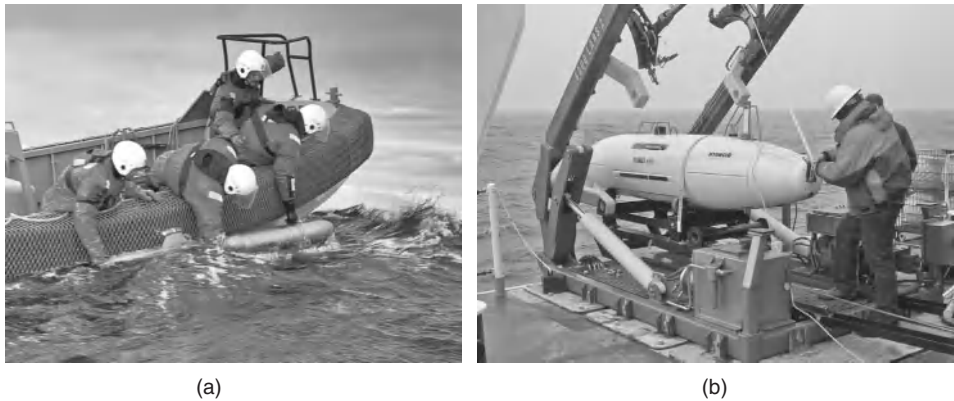
Fig. 3.4 Autonomous underwater vehicles (AUV) (a) Gavia coastal AUV system with primarily imaging sensors (courtesy of Teledyne Gavia) (b) Remus 6000 large oceanographic AUV system with near-bottom imaging capabilities (credit: Hydroid). (For a colour version of this figure, see Plate 3.2.)
