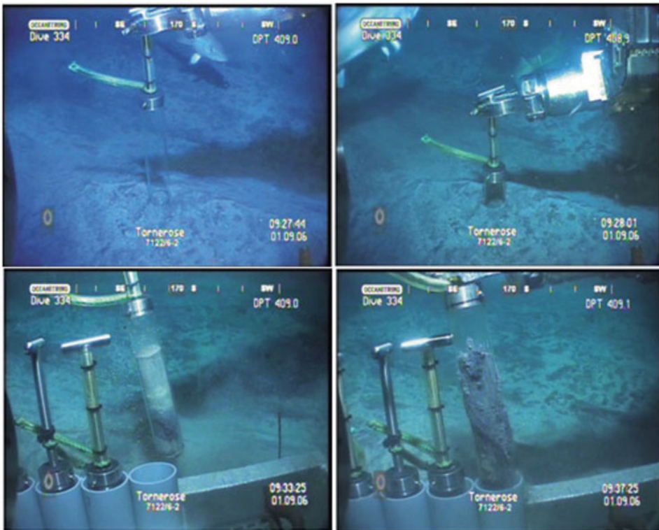
Plate 7.5 Remotely Operated Vehicle (ROV) push cores in use in the Barents Sea. (Images © SERPENT.)
