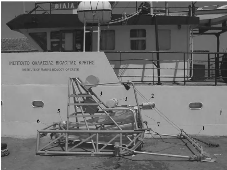
Fig. 5.4 The Towed Trawl Simulator Sledge (TTSS2; Koulouri et al. , 2003). 1, Ground rope; 2, opening–closing mechanism; 3, electronic controller; 4, television camera; 5, collectors; 6, odometer; 7, superimposed nets.
