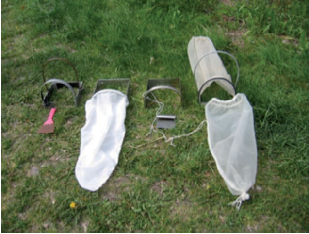
Fig. 9.5 Frames used within the Swedish monitoring programme and a picture of some modifications (second from left is the original). Four different designs of 'Kautsky' frame used in different Baltic laboratories (recommended by HELCOM COMBINE Guidelines).
