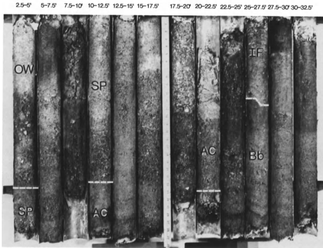
Figure 4.13. Core photograph of wave-dominated inlet-fill sequence from Core Banks, North Carolina. The inlet-fill sequence is approximately 8.0 m (25.75 ft) thick, and comprises inlet-floor (IF), active-channel (AC), and spit-platform (SP) facies. The sequence fines upward, consists of an
