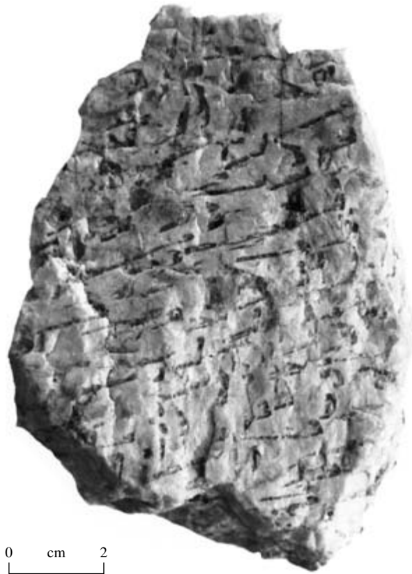
7.20 Graphic texture in hand sample of graphic granite. The scattered quartz grains in a single-crystal host of perthitic alkali feldspar resemble poikilitic texture. However, the quartz grains are more or less uniformly spaced and are not randomly oriented. They are all crystallographically continuous, as may be verified by their optical continuity viewed in thin section under cross-polarized light, and grew simultaneously with the alkali feldspar as an intergrowth .
