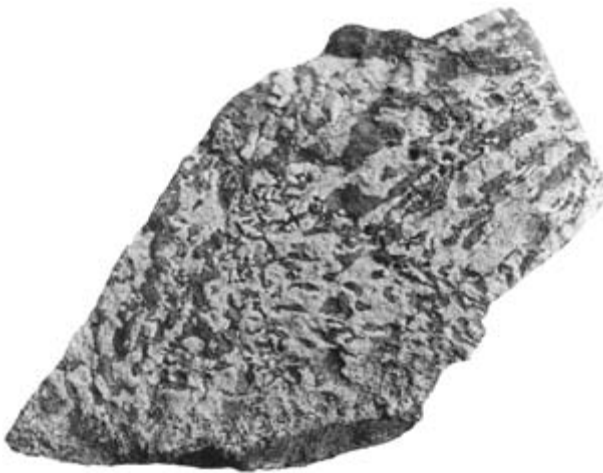
14.21 Metasomatized graphic granite in wallrock adjacent to a carbonatite dike (Figure 13.40). Quartz grains have been replaced by fine-grained aggregates of sodic amphibole produced by reaction with highly alkaline solutions expelled from the carbonatite magma.
