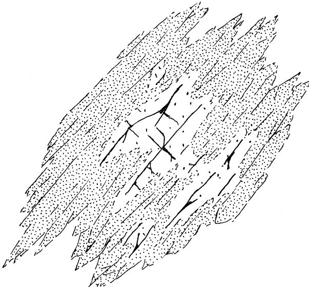
14.7 Overgrowth and replacement of primary magmatic clinopyroxene by a bundle of subparallel amphibole needles. Development of this specific texture is called uralitization but is a type of epitaxy or epitaxial growth in which a secondary phase nucleates and grows on a crystalline substrate that has a similar atomic structure and influences the orientation of the overgrowth. In this case, amphibole and clinopyroxene are both chain silicates.
