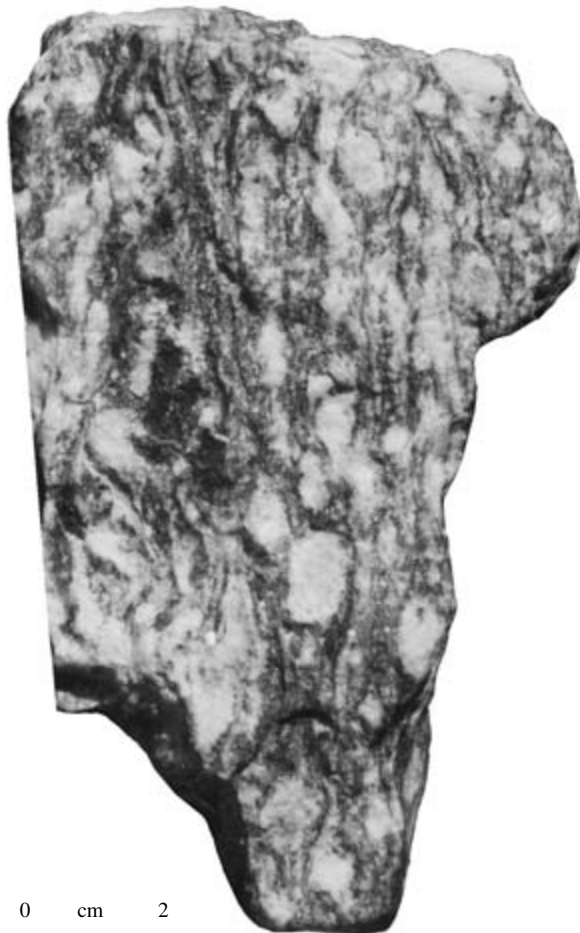
15.7 Augen gneiss. Ovoidal or eye-shaped megacrystals of alkali feldspar in biotite-rich lepidoblastic matrix. Rock breaks across foliation.
