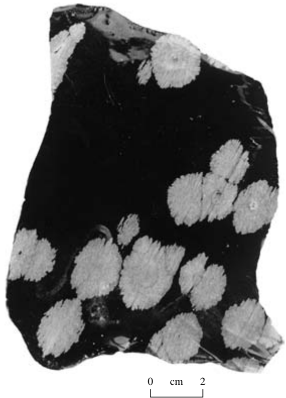
7.6 Spherulitic texture in high-silica rhyolite obsidian. Spherulites are spherical to ellipsoidal clusters of radiating fibrous alkali feldspar and a polymorph of SiO_2 , here in a black glassy matrix. Faint, relict flow layering that extends from lower left to upper right is accentuated in the spherulites in this hand sample, indicating their growth after active flow of the magma. Individual spherulites in volcanic rocks can range in diameter from less than 1 mm to 1 m or so. A phenocryst may be located at the center of the spherulite, where, in the original glass or drastically undercooled melt, it allowed heterogeneous nucleation of crystals to occur. Spherulites are secondary devitrification features, not phenocrysts .
