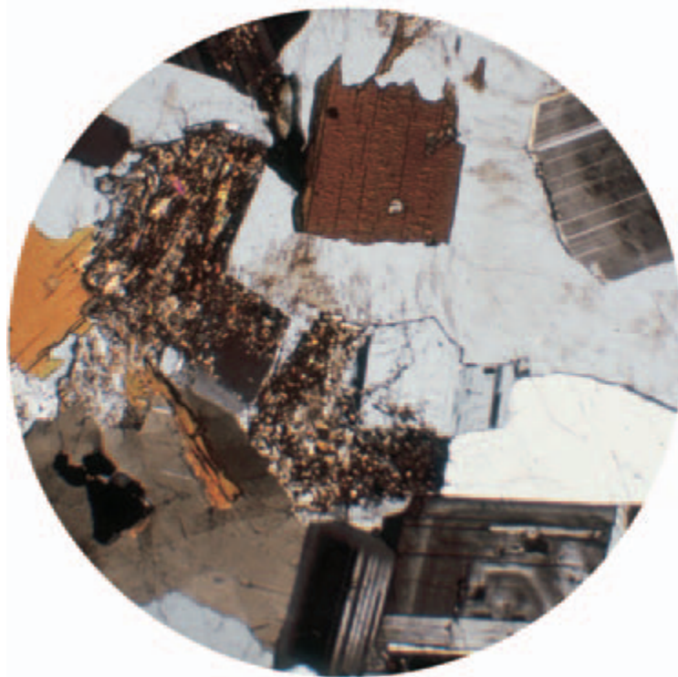
IV Photomicrograph of an altered subsolvus granite in which primary high- T magmatic plagioclase and biotite have been partially decomposed by subsolidus breakdown reactions. (a) Plane-polarized light showing dark brown biotite partially replaced by green chlorite in thin lenses parallel to (001) and plagioclases on left replaced by a fine-grained phyllosilicates and possibly an epidote mineral. Also note clay-altered alkali feldspars that have a “turbid” appearance. (b) Cross-polarized light of same view showing highly birefringent replacement particles in upper plagioclase and euhedral form of fresh plagioclase against alkali feldspar and quartz in lower part of view. This contrast in euhedralism is interpreted to have originated as alkali feldspar and quartz crystallized near the solidus from a melt lying between the higher- T plagioclase crystals. Note undulatory extinction in strained quartz (lower left).
