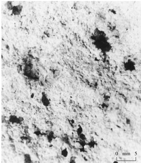
7.25 Vuggy fabric in felsitic aphanitic rhyolite. Collection of exsolved volatiles into irregularly shaped pockets in a highly crystalline matrix produces vugs. They are commonly lined with euhedral vapor-phase crystals that grew freely in the entrapped volatile fluid. Vapor-phase precipitates include quartz (seen here), specular hematite, and, in some peraluminous rhyolites, topaz and Fe-Mn garnet.
