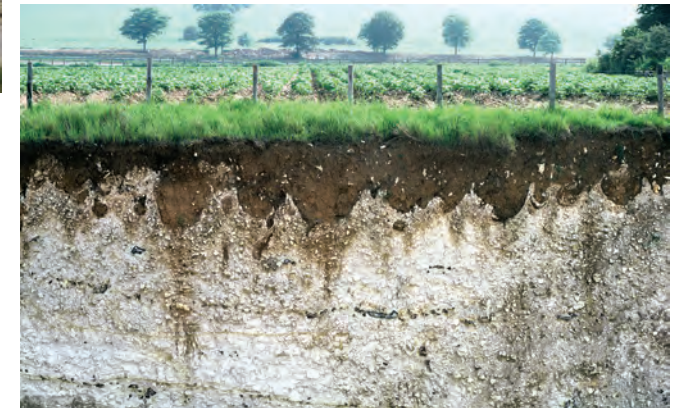
A cryoturbated interface between chalk and a residual clay soil formed by periglacial ground ice heave that has been complicated by later dissolution of the chalk.
