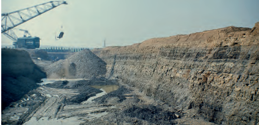
Coal Measures in an opencast mine, with horizontal, dark grey mudstones and buff sandstones above a coal seam at floor level; this method of mining is economical where overburden is less than about 20 times the seam thickness.
