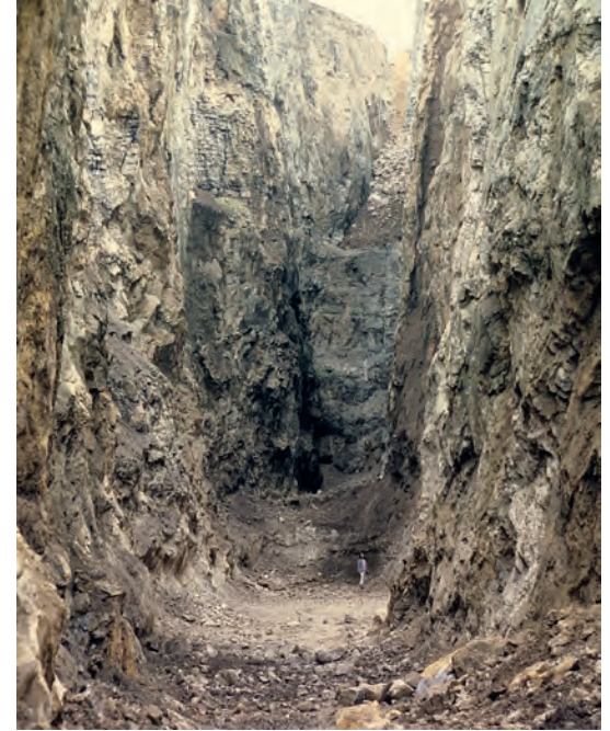
A deep open mine on a vertical mineral vein, with abandoned faces that are higher than would be acceptable in any modern quarry.
