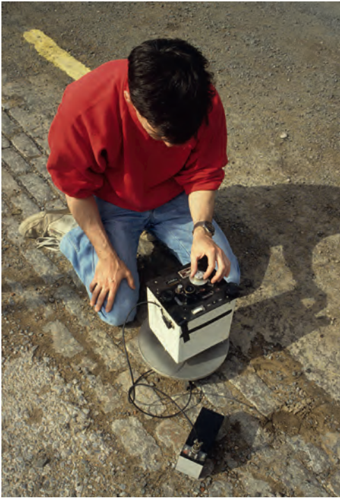
[above left] Microgravity survey searching for negative anomalies that indicate the presence of mined cavities at shallow depth in sandstone.
