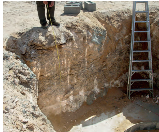
[near right] A trial pit provides the best information on the top few metres of the soil profile, but a pit requires support struts if it is taken any deeper.
