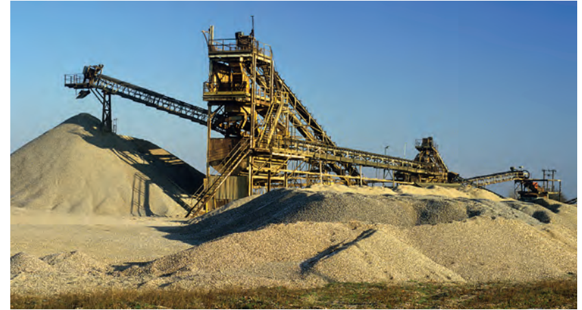
Screening plant and stockpiles at a pit producing aggregate from alluvial gravel.
