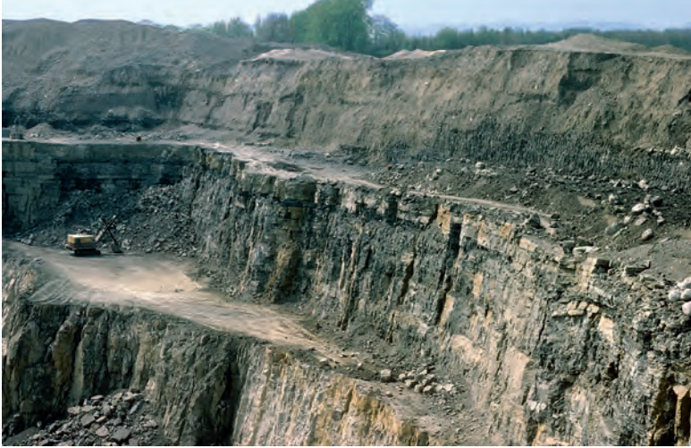
[top left] The upper bench of an aggregate quarry lies on the top of the strong limestone, and the upper face is an overburden of shales and glacial till that has to be cleared.
