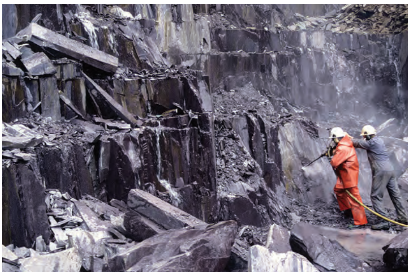
Best-quality slate being quarried in North Wales, where the cleavage is nearly vertical and is crossed by at least three sets of fractures.
