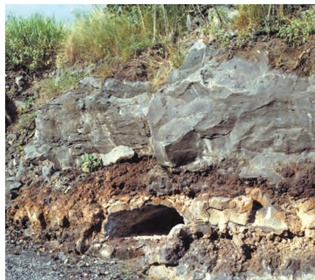
Variation in basaltic ground, in a road cut in Hawaii, with a solid, strong lava overlying a weaker lava with a rubbly aa top and an open lava tube inside it.
