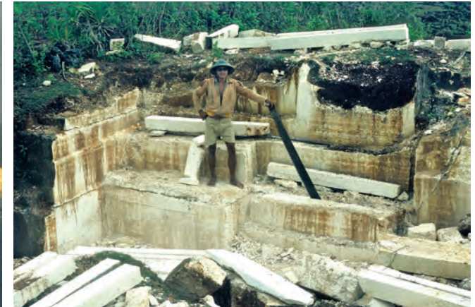
A weak, chalky limestone is sawn by hand into blocks that case-harden by re-deposition of carbonate in the surface layers after a few weeks of exposure and drying.
