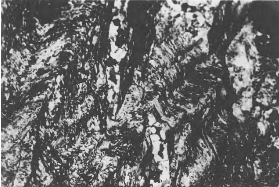
Fig. 2. Crushing and partial dislocation of quartz
