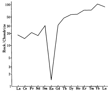
Fig. 4. Chondrite-normalized REE pattern of the Gejiu tin-bearing granite
