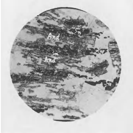
Fig. 8. Cassiterite alternating with andalusite (And), forming striped distribution (linearly polarized light, 30x)
