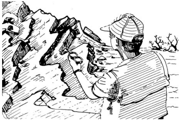
Fig. E.1 Sighting with a compass along a line of outcrop to obtain an averaged strike direction. Caution – the line of sight must be horizontal
