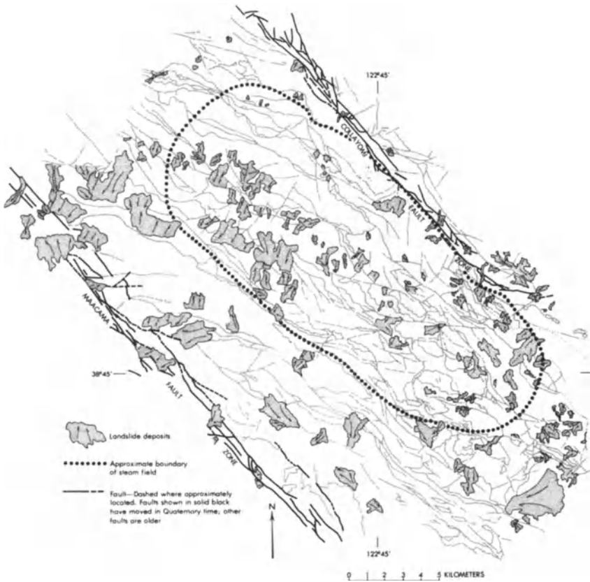
FIG. 2.2. Map illustrating landslides and faults in The Geysers geothermal field, California, USA. After McLaughlin, R. J., 1978. Preliminary Geologic Map and Structural Section of the Central Mayacamas Mountains and The Geysers Steam Field, Sonoma, Lake and Mendocino Counties, California . US Geol. Surv. Open-file Rept 78-389 (2 sheets), scale 1:24 000. Reproduced from Fig. 7.2 in Chapter 7, Environmental aspects of geothermal development, by M. D. Crittenden Jr, in Geothermal Systems: Principles and Case Histories , ed. L. Rybach and L. J. P. Muffler, 1981, by permission of the publishers, John Wiley & Sons Ltd.
