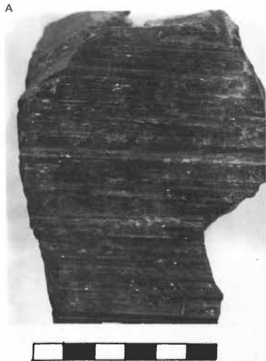
Figure 2.6 A. Hand specimen showing slickenside striations on a fault surface. Scale bar, 6 cm.
