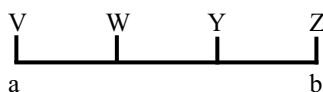
Figure 12.1 Chemography for the two-component system a-b with phases V, W, Y, Z. The topology for this system is shown in Figures 12.2 and 12.3.
