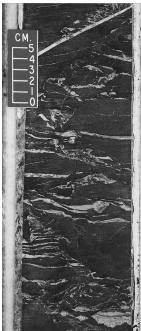
Fig. 5.15. Core photograph of small-scale injection features showing sand-filled microfractures in mudstone host. Note small-scale normal faults. Eocene, North Sea.
