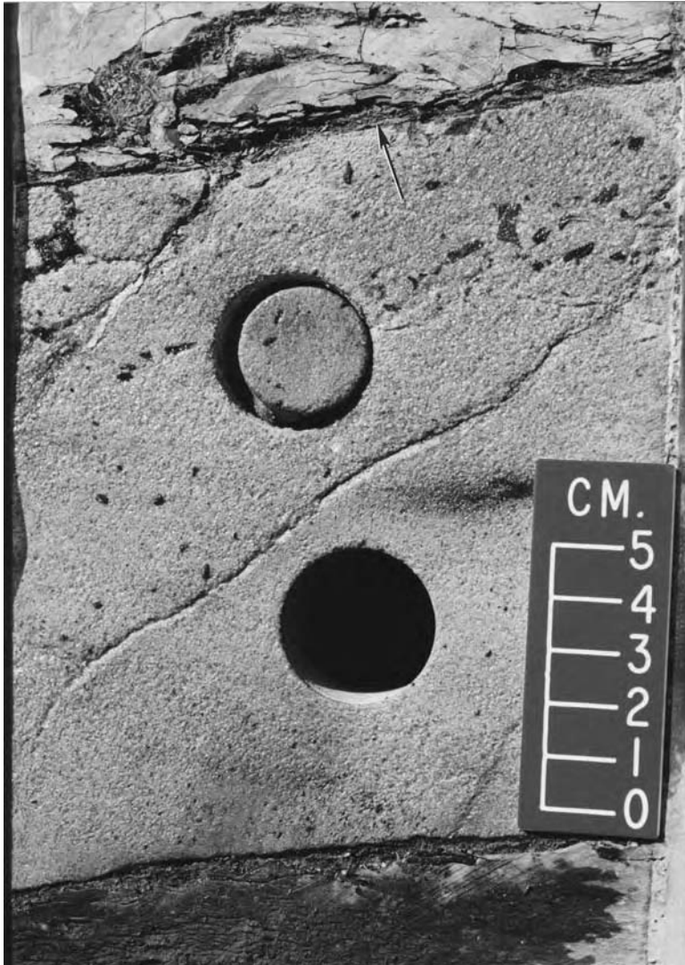
Fig. 5.6. Core photograph of a sandstone injection showing pulverized matrix at the margin with mudstone host (arrow) above. Note scattered mudstone chips near the top of injected sandstone. Eocene, North Sea.
