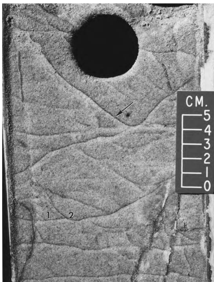
Fig. 5.1. Core photograph showing water-escape dish structures by liquidization in fine-grained, well-sorted sand. The arrow shows a concave-up (dish structure) color couplet with left wing dipping at 45^\circ from the core horizontal due to deformation. Note cross-cutting relationship between two dish structures in which an earlier formed dish structure (1) has been terminated by a later one (2). Eocene, North Sea.
