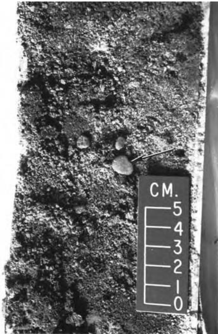
Fig. 3.13. Core photograph showing floating quartz granules (arrow) in fine-grained sand implying flow strength. Eocene, North Sea.
