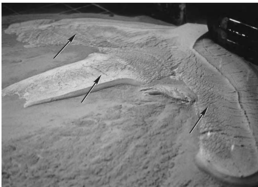
Fig. 12.3. Flume experiments of debris flows showing tongue-like sediment (arrows) in front of the channel mouth. Note sharp and irregular fronts (i.e., snouts). Flow from upper right to lower left. (Photo courtesy of J. Marr (St. Anthony Falls Laboratory, University of Minnesota).)
