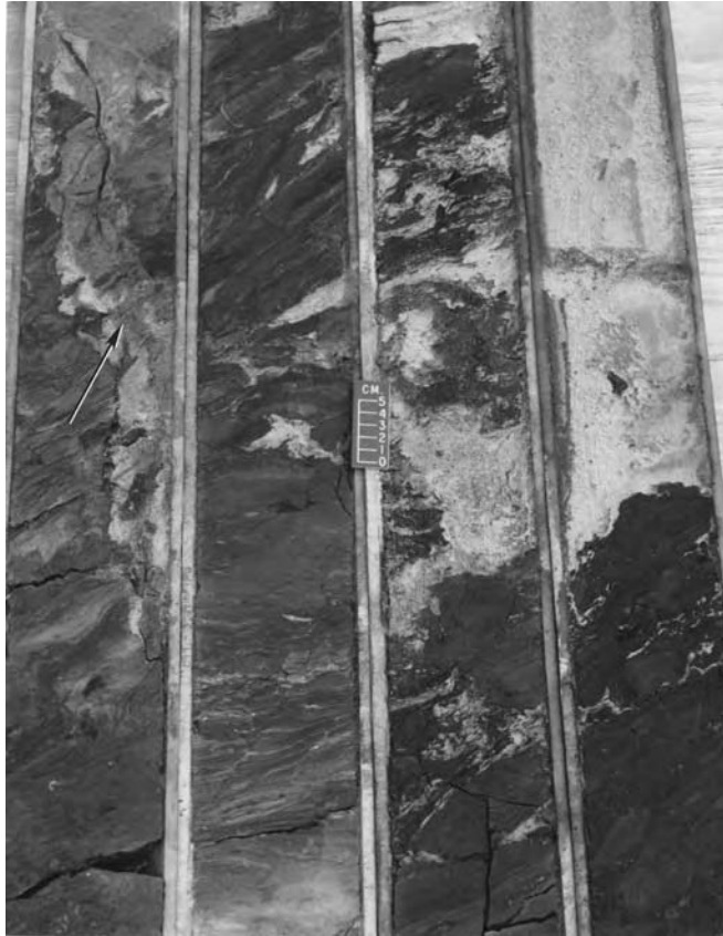
Fig. 5.2. Core photograph showing a vertical pillar of sand (arrow) cutting across mudstone. Lower left is bottom and upper right is top. Pliocene, offshore Nigeria.
