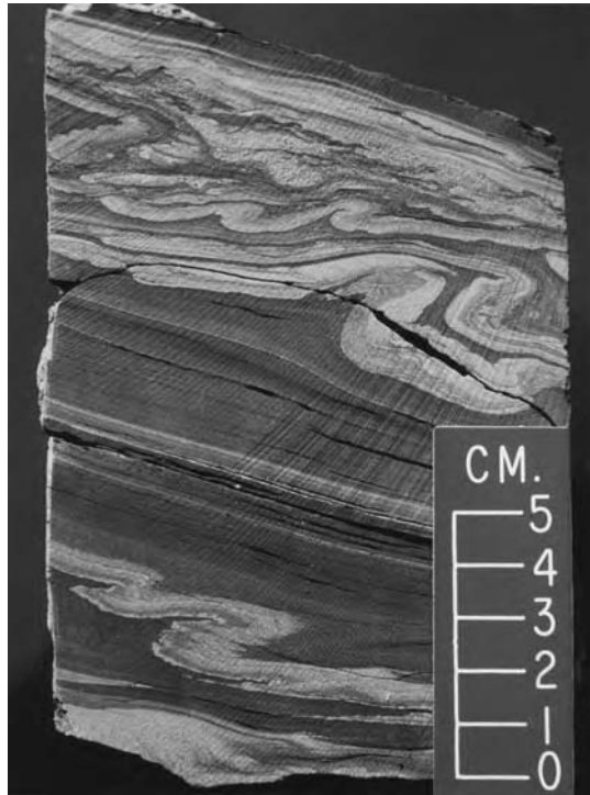
Fig. 3.7. Core photograph showing alternation of contorted and uncontorted siltstone (light color) and claystone (dark color) layers of slump origin. Paleocene, North Sea.
