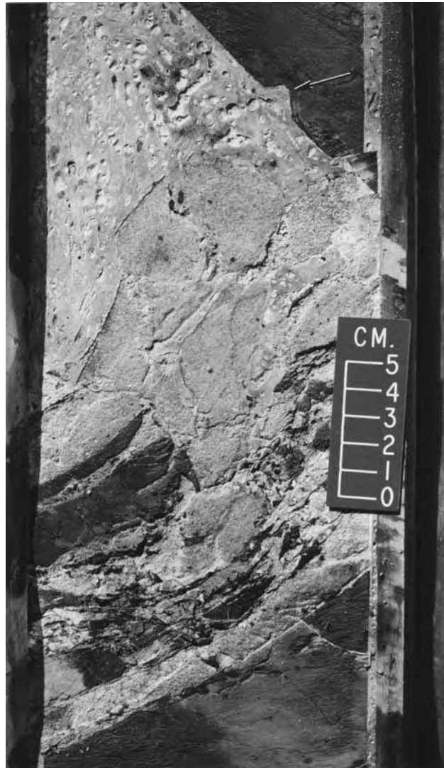
Fig. 5.5. Core photograph of a sandstone injection showing indented margin (arrow) with mudstone host. Note mudstone chips near the bottom of injected sandstone. Eocene, North Sea.
