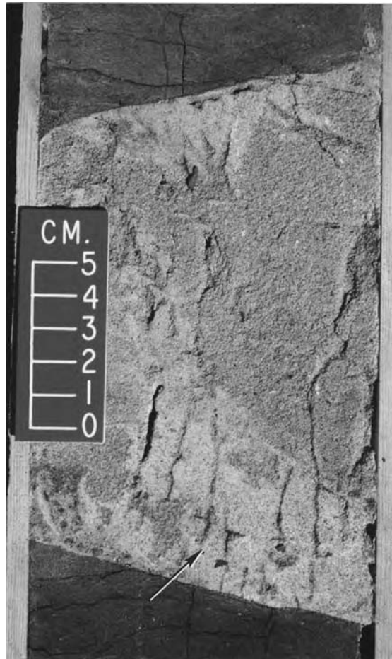
Fig. 5.3. Core photograph showing horizontal sandstone injection with razor-sharp margin into mudstone host. Note vertical shear fractures (arrow) within the sill. Also note termination of depositional laminae in mudstone above and below by the injection. Although sandstone sills are concordant features, they terminate depositional laminae (i.e., horizontal layers in mudstone) and thus qualifying to be discordant ‘dikes’ as well. Eocene, North Sea.
