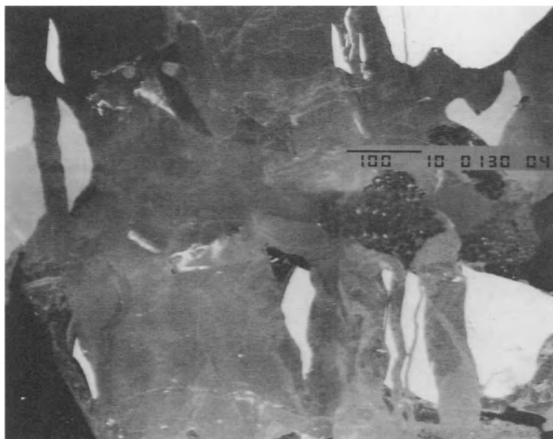
Fig. 7. Complex grain/cement intergrowth in a crack-seal fracture fill. Repetitive fracturing has transported highly angular slivers of bright luminescing detrital quartz relatively large distances across the fracture. Luminescence variations that suggest complex intergrowths of different generations of authigenic quartz are indicative of fracture movement synchronous with quartz precipitation leading to fracturing and overgrowth of the earlier-formed cement. Frontier Formation, Wyoming. Scale bar is 100 \mu\text{m}
