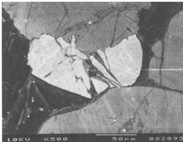
Fig. 6. Fractures propagating from region of maximum curvature along sutured grain boundary. Field of view is entirely quartz. Breathitt Formation, Pennsylvanian, eastern Kentucky
