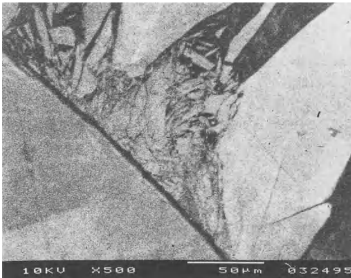
Fig. 3. Crushed grain boundary from the subsurface Frio Formation Texas Gulf coast. Field of view is uniform quartz with only minor visible microporosity. Dark luminescing quartz is authigenic whereas the detrital grains and their fragments are bright
