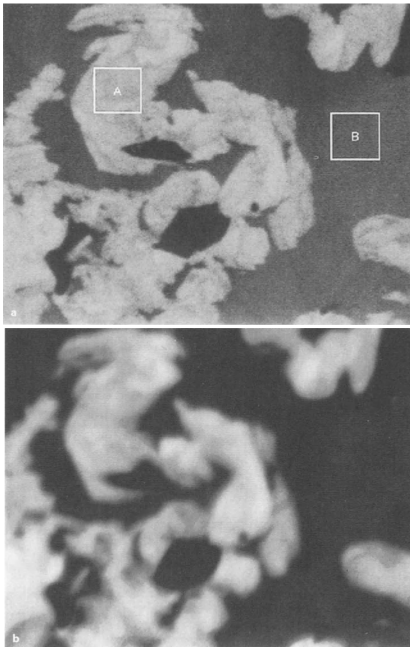
Fig. 24a,b. Scanning CL images measured with a 5 keV (a) and 15 keV (b) incident energy from an area exhibiting bright luminescent spots at the surface of the natural zircon. Note the change in the spatial resolution as a function of the accelerating voltage (see Sect. 4.4)
