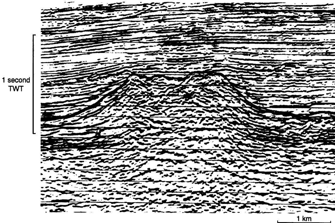
Figure 2.11. A 'pinnacle' type carbonate platform from the Miocene of offshore Philippines. It is impossible to break out different systems tracts from seismic data alone in this example, which shows continuous gradual backstepping and confused internal seismic character. The top of the platform is very rugose which represent karsting or the break-up of the platform into several small pinnacles prior to drowning. Used with permission of Blackwell Science.
