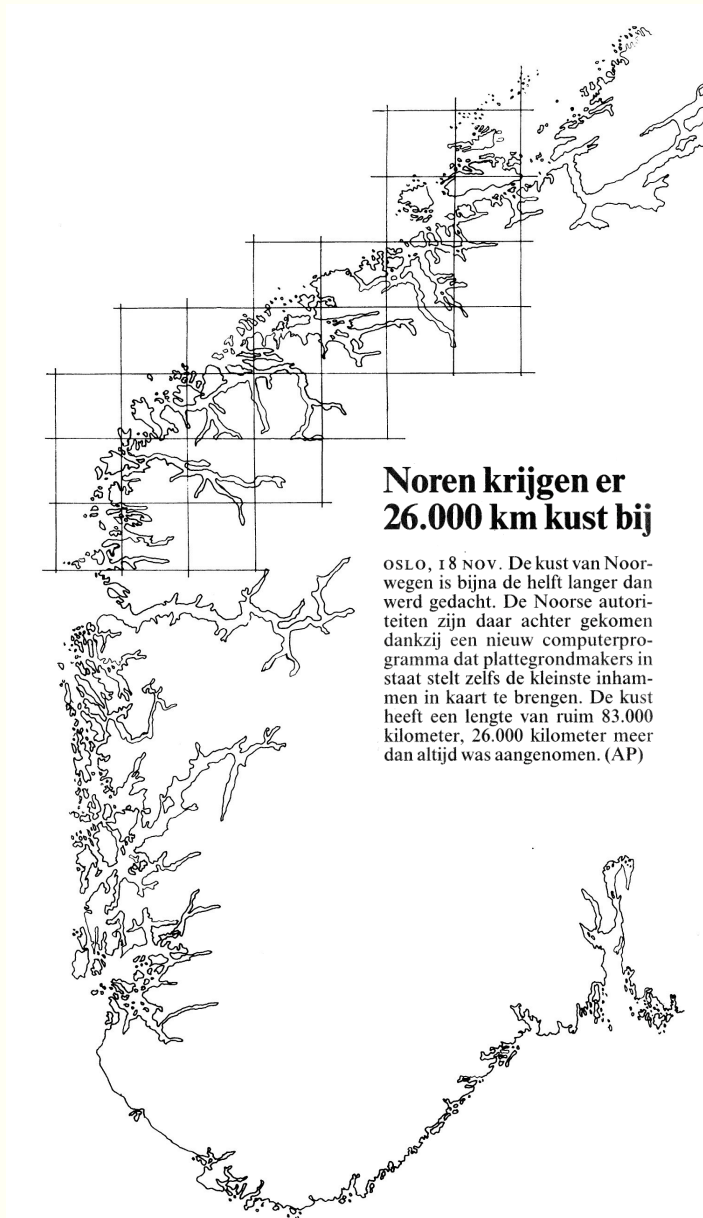
Fig. A.3. — Coastlines were among the first natural phenomena whose fractal nature was recognized. Here we see part of the coast of Norway. The clipping from a Dutch newspaper reports that the Norwegian coast has become 26,000 km longer because it was surveyed in finer detail. Based on Feder (1988).
