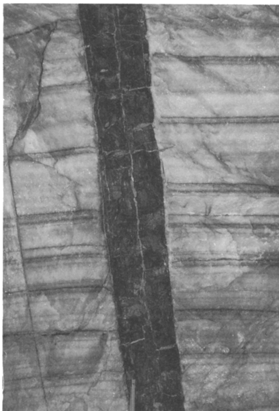
Fig. 3.1 Outcrop 1-ug in K1H. The massive, 6.5-cm-wide basanite dike exhibits comparatively few fissures and cracks. The light-colored patches in the dike are fracture surfaces covered by salt dust. Smaller gas cavities are seen on both sides of the dike.
