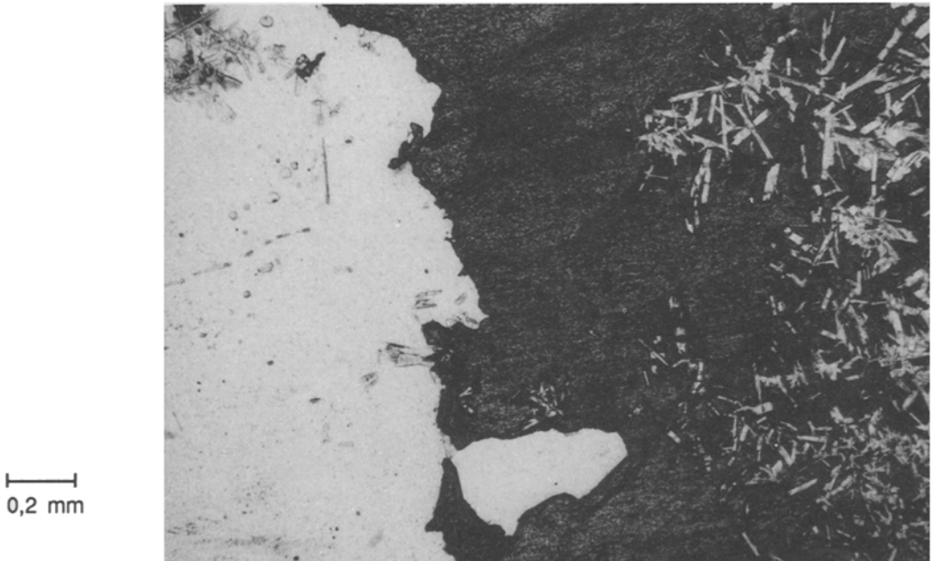
Fig. 6.2 Outcrop 60-ug in K1H. Native sulfur contains inclusions of fine needles of anhydrite.
