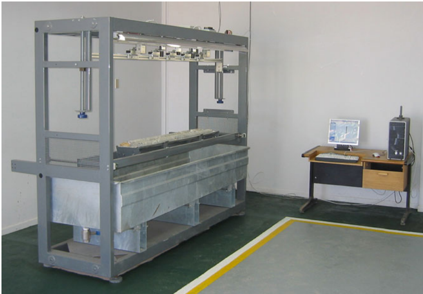
Fig. 4.17 Frame holding four digital cameras of high resolution used for photographing core at the Escondida copper mine, Chile
