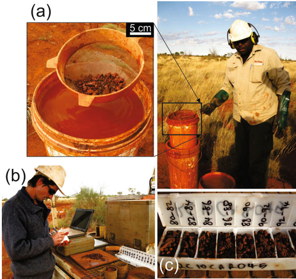
Fig. 4.31 Processing and documentation the rock chips recovered by RC drilling: (a) washing rock chips from clay and dust; (b) petrographic logging of the rock chips;
