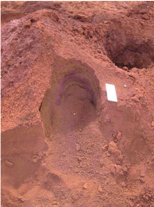
Fig. 4.26 Example of the blasthole sampling when bottom of the pile is not correctly represented in the collected sample
