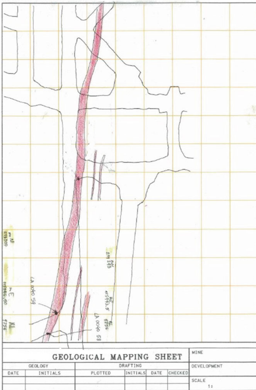
Fig. 3.9 Mapping sheet prepared for geological mapping at the Perseverance nickel-sulphide underground mine, Leinster, Australia. Outlines of the mine workings were
