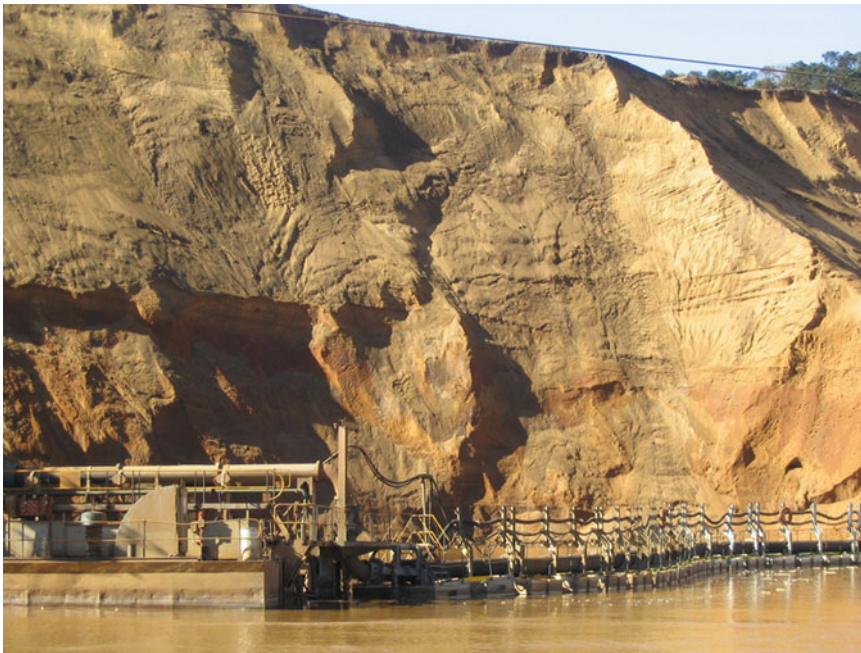
Fig. 2.13 Dredging at the Richards Bay titanium sands deposit, South Africa
