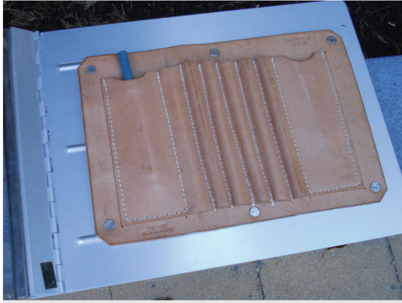
Fig. 3.10 Mapping sheets holder with attached pencils sheath for underground mapping
