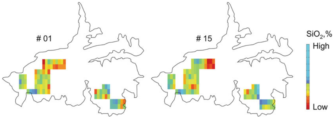
Fig. 28.3 Two equiprobable realisations (#01 and #15) of the SGS model of the \text{SiO}_2 (%) grade built using 200 \times 200 m data and averaged to the panels of 230 \times 450 \times 3.5 m. Panel's size is equal to the monthly production plans
