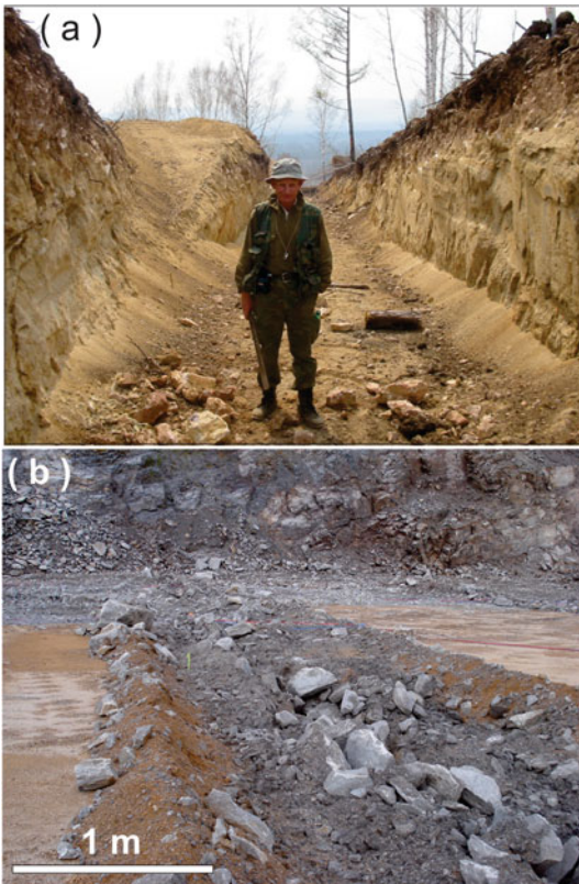
Fig. 5.6 Examples of trenching in mining industry: (a) exploration trench dug by dozer, Bystrynsky Cu-Au project, Siberia, Russia; (b) trench ripped by a dozer ripper
