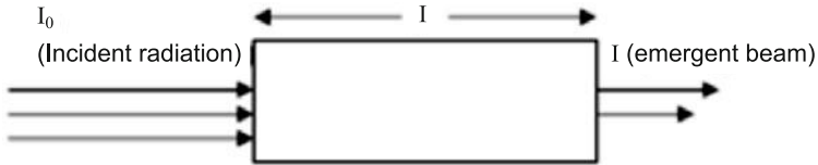
Fig. 13.42: Absorption of radiation while passing through a medium.
