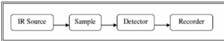
Fig. 13.48: Block diagram of IR analytical technique.
