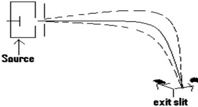
Fig. 13.25: A cylindrical electrostatic sector energy filter.
