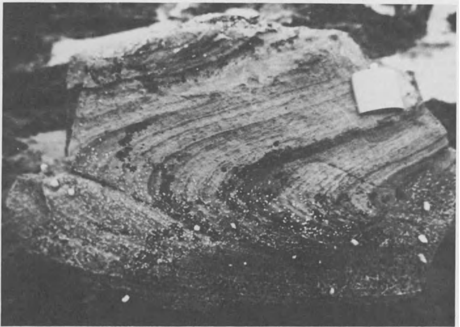
Figure 10.12a and b Slump bedding in interlaminated sands and shales within the Helmsdale boulder beds, Kintradwell, Sutherland. These features indicate deposition on a slope.
