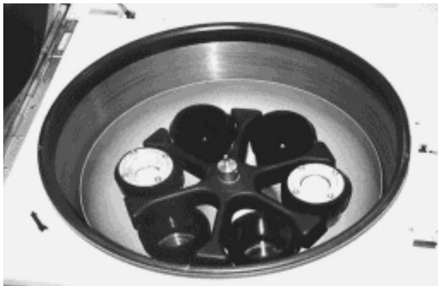
Figure 3.46 Small scale medical centrifuge rotor assembly with six swinging type buckets (after Khanzode et al. , 2002).
