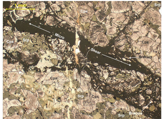
Plate SP-15 Micro-shear in spinel Iherzolite containing pulverised and brecciated grains of clinopyroxene and serpentine (96/80b)
