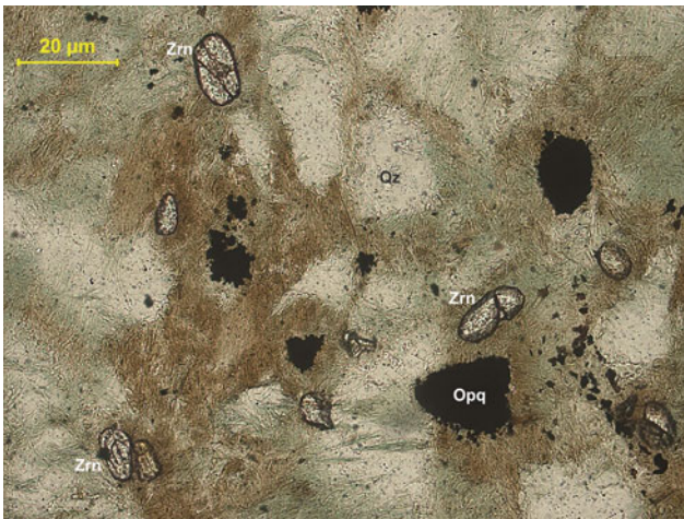
Plate Py-24 Ignimbrite with angular and corroded quartz, skeletal and disseminated opaque, and zircon set in a groundmass containing green chlorite admixed with fine brown glass (LKM5/89-1)
