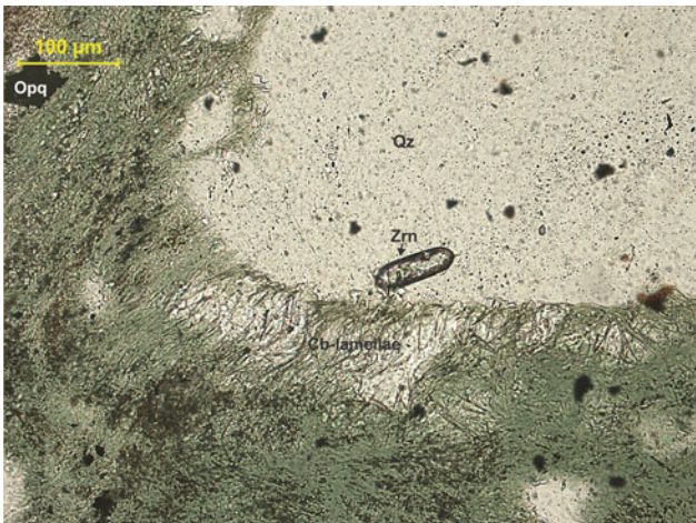
Plate Py-25 Magnified view of inclusion of zircon in sub-rounded quartz showing simple pressure fringes with growth of calcite fibres (carbonate-Cb) perpendicular to quartz in ignimbrite. The groundmass is made of chlorite (LKM3/89-6)
