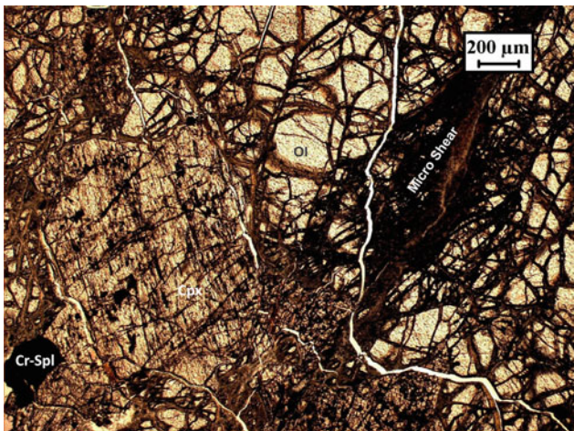
Plate SP-14 Spinel Iherzolite with micro-shear containing olivine and clinopyroxene with streaks of opaque along the cleavage (K72-8)
