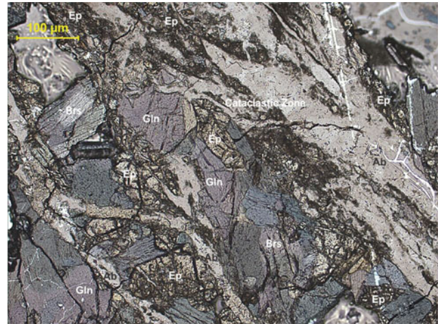
Plate Ec-14 A cataclastic zone in eclogite showing multiple veins of albite cutting through brecciated clusters of epidote, glaucophane and barroisite (77/80-5)
