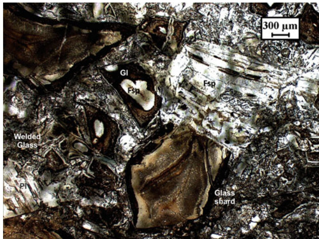
Plate Py-9 Welded crystal-vitric tuff containing feldspars rimmed by glass and shards. Channels and grooves inside a cusped glass shard probably represent escape routes for volatiles upon consolidation (17/79-1)
