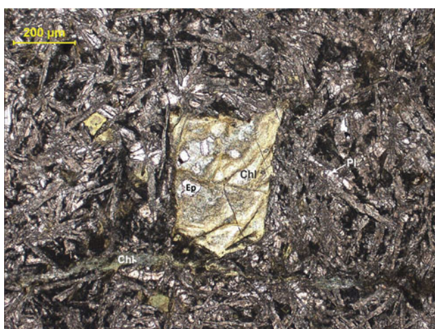
Plate V-1 Pseudomorph of chlorite + epidote after olivine phenocryst in porphyritic olivine basalt. The fine-grained groundmass shows an intersertal to intergranular texture (230/79-2)
