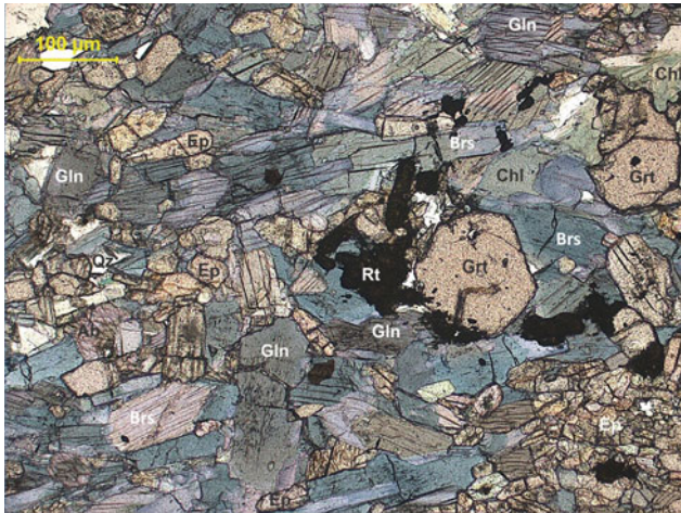
Plate Gln-23 Epidote-garnet-glaucophane-barroisite schist showing a granoblastic texture with minor garnet, phengite, rutile and late albite (139/79-1)
