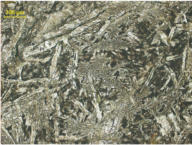
Plate V-9 Plagioclase-phyric basalt showing intergranular to intersertal texture. It consists of skeletal plagioclase and pyroxene altering to chlorite and iron oxides (230/70-1)
