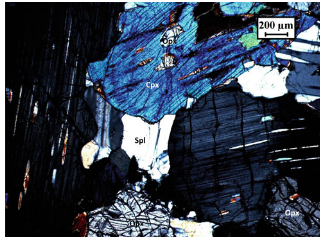
Plate G-18 Gabbronorite 169/80-1 between crossed polars showing exsolution lamellae in clinopyroxene (169/80-2)
