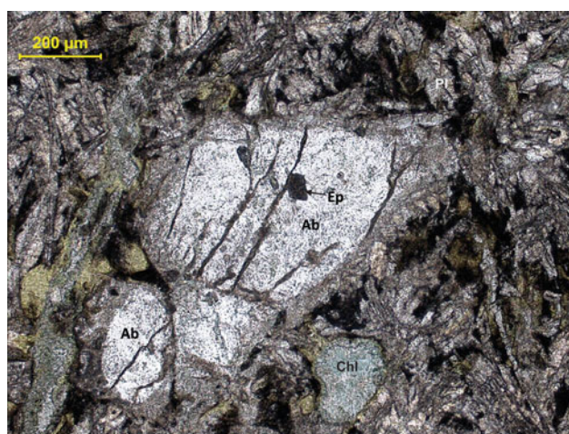
Plate V-3 Phenocryst of albite in basalt showing longitudinal cracks filled with secondary chlorite. The groundmass contains acicular clinopyroxene and green chlorite rimmed by epidote (230/79-4)
