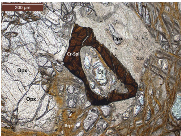
Plate SP-6 Skeletal spinel containing a large inclusion of serpentinised olivine. The prismatic grain of greyish clinopyroxene on right contains inclusions of orthopyroxene (R-16-1)
