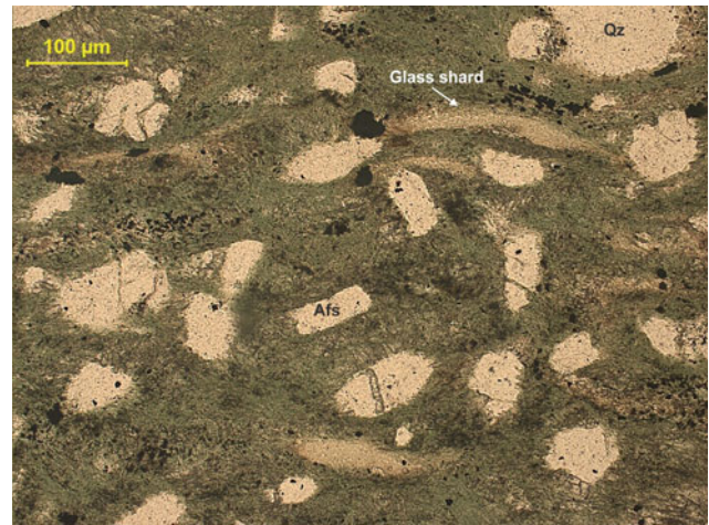
Plate Py-22 Ignimbrite showing devitrified glass shards with diffused outlines, poorly sorted and angular quartz, feldspar and opaque grains embedded in chloritic groundmass. Random orientation of minerals indicates crystallisation in a plastic flow by rheomorphism (LKM3/89-5)
