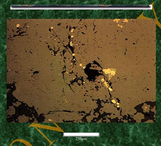
Sphalerite (grey), the main phase, encloses irregular chalcopyrite (yellow, top right) and fine chalcopyrite inclusions (centre) but is essentially free of chalcopyrite disease. Small euhedral pyrite crystals (pale yellow-white, centre) lie in a discontinuous veinlet cutting sphalerite. A triangular inclusion of tennantite (green-blue, centre right) is associated with chalcopyrite and two pyrite crystals. Quartz is dark grey, black areas are polishing pits.
