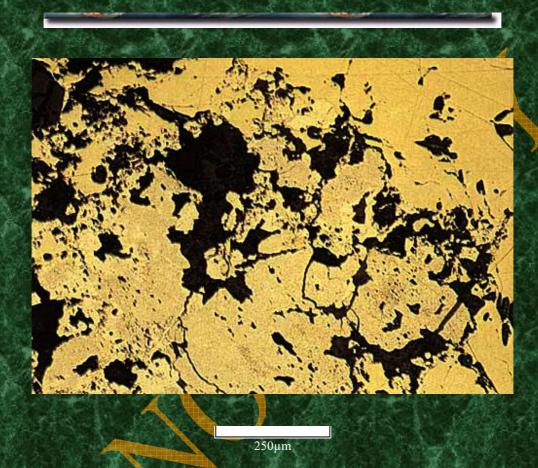
Chalcopyrite (yellow, right) surrounds poorly crystalline, fine-grained pyrite (brown, bottom centre) which has well crystalline margins (pale yellow-white, centre). The fine-grained nature of pyrite lowers its reflectance and gives a characteristic brown surface colour. The fine pyrite could be primary or altered pyrrhotite, but here it is probably primary. The gangue phases (dark grey) are silicates.
