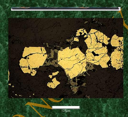
Euhedral pyrite (light yellow, centre) is fractured and surrounded by aggregates of finegrained, often botryoidal, haematite (light green-grey, centre left). The differences in reflectance and surface colour (bottom centre) between the core and margin of the haematite aggregates are due to variations in grain size of individual haematite crystals. The coarser crystals on the margin have a slightly higher reflectance. Quartz (dark grey) is the gangue.
