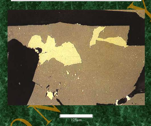
Sphalerite (grey) shows a slight variation in reflectance and very faint reddish internal reflections (both very difficult to see) due to submicroscopic inclusions of tetrahedrite (right centre). Coarse-grained tetrahedrite (green-blue, centre left) is also present within sphalerite as is chalcopyrite (yellow, bottom left). A minor amount of galena (white) lies in the gangue between sphalerite crystals (bottom right).
