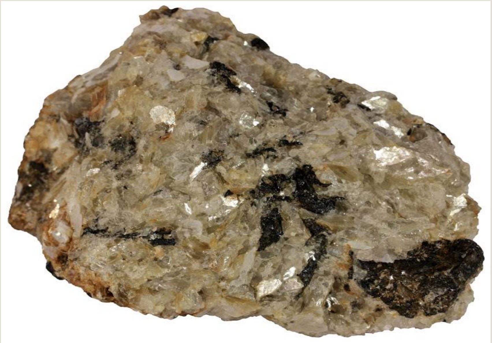
Fig 7: Greisen sample with mica and cassiterite ( \text{SnO}_2 )
