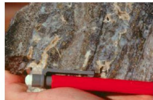
Photo 6. Telescoped low sulphidation mineralization with pyrite, base metal sulphides and opal from Tavatu
