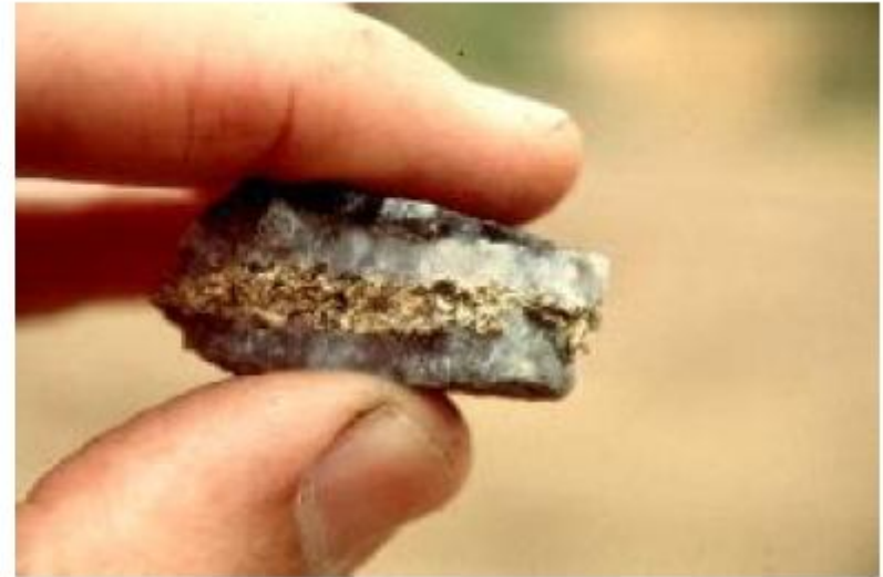
Photo 18. Bonanza gold grade epithermal quartz gold-silver style mineralization comprising gold fill of an open quartz vein, Edie Creek.
