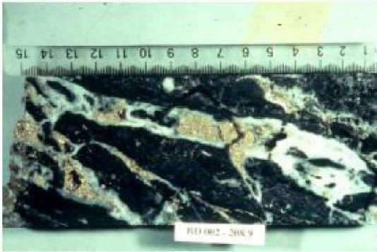
Photo 1. Quartz-sulphide gold ± copper style mineralization from Bilimoia (Corbett et al 1994) containing early quartz and later coarse crystalline pyrite.
