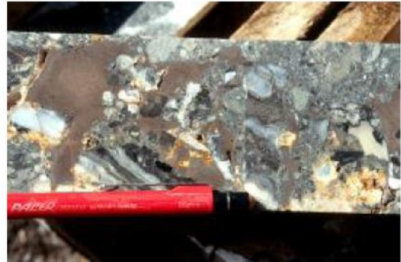
Photo 24. Toka Tindung eruption breccia with sinter and wood fragments in a strongly silicified matrix
