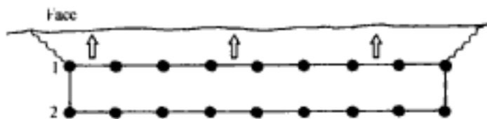
Figure 5.32. Double row shot instantaneously (Hagan & Mercer, 1983).
