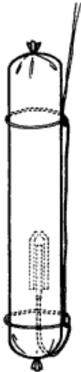
Figure 8.42. Attaching an electric blasting cap to a cast primer. DuPont Blasters Handbook, 1977.
