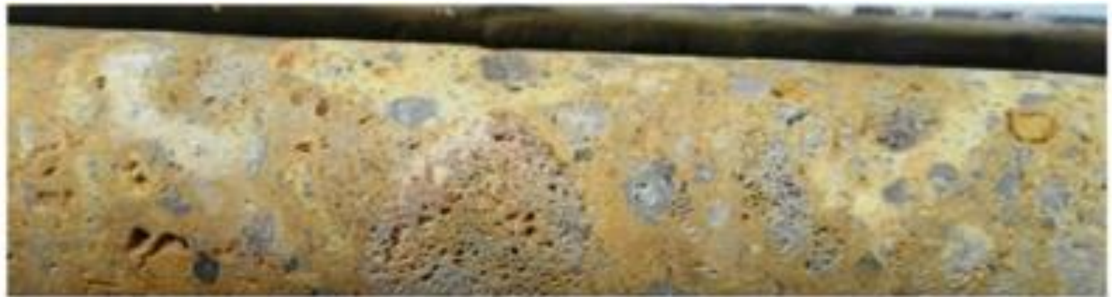
414m (2.54 g/t Au & 1.1 g/t Ag), "Yellow" polymict hydrothermal breccia jarosite-alunita-barite-filled matrix with sub angular vuggy silica altered fragments
