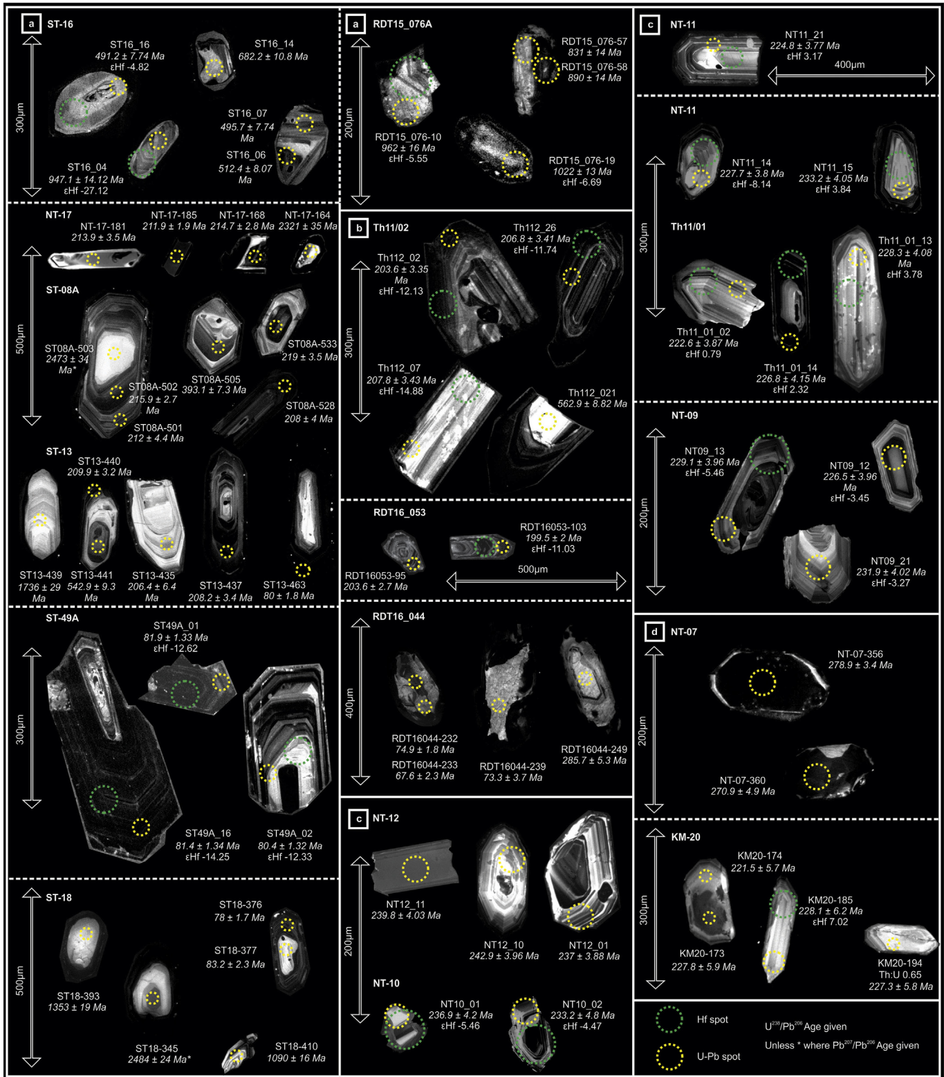
Fig. 2. Representative cathodoluminescence images for all granitoid rocks sampled in Thailand. U–Pb laser, Hf spots shown. The age given for each spot is the U^{238}/Pb^{206} age, unless marked with an asterisk (*) indicating that the Pb^{207}/Pb^{206} Age is given. Individual spot \epsilon Hf(t) values are given.
