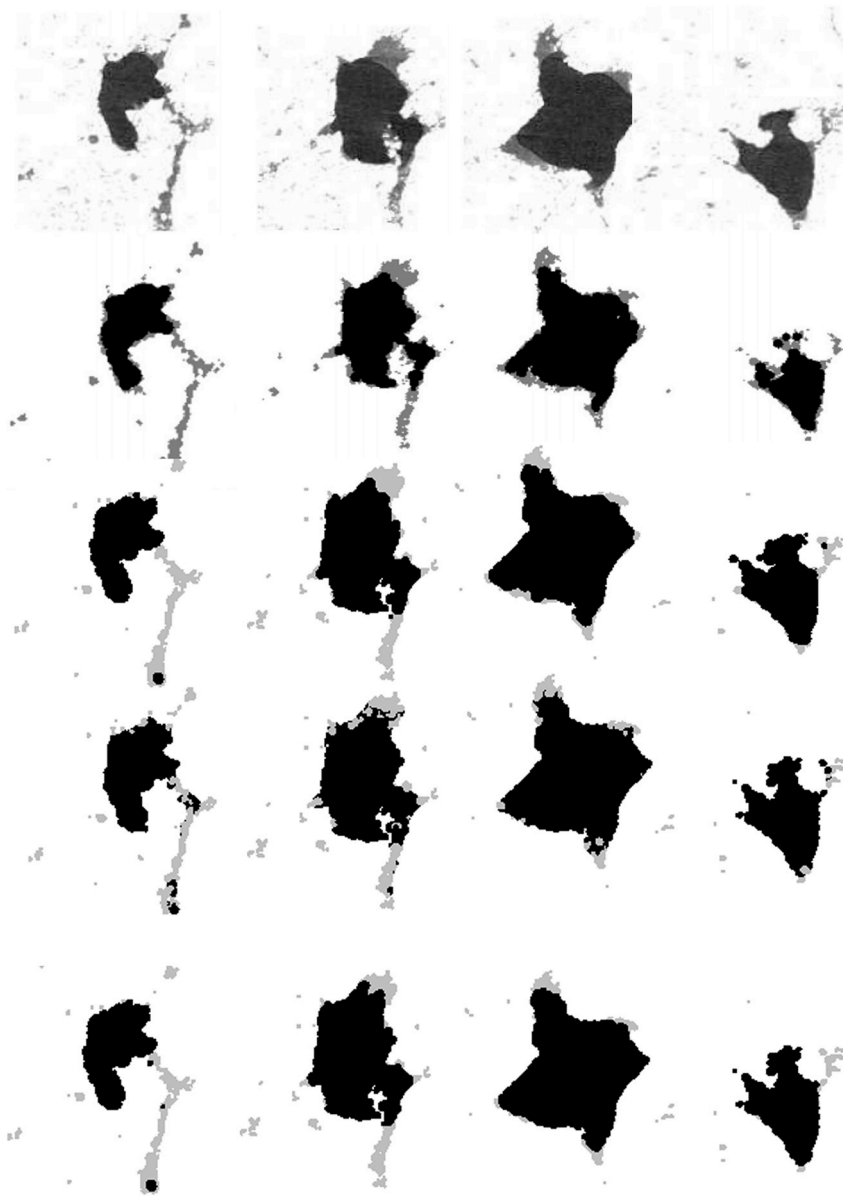
Fig. 6. Comparison between segmented SR- \mu CT data (first row) and model predictions of the air-water distribution in the connected pore space of ROI p1bkk03a at different vertical sections z = 18, 24, 34, and 65 (from left to right). The water saturation index of the pore is 0.20 . Solid phase is in white, water is in light gray, and air is in black. The second row corresponds to predictions using spherical balls, whereas the third, fourth, and fifth result from modeling with ellipsoids defined on the basis, respectively, of the minimal radius (3rd row), maximal radius (4th row), and mean radius (5th row). To drain ellipsoids, the threshold diameter is taken as 73.6 \mu\text{m} according to Pot et al., (2015) .
