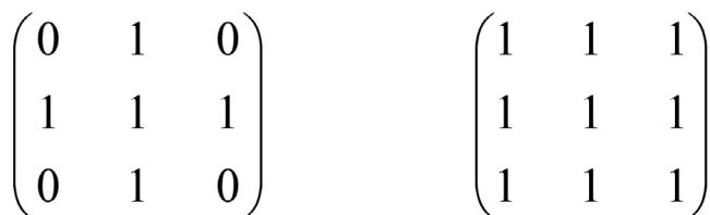
Fig. 1. Matrices for 4 (left) and 8 (right) connected components.
