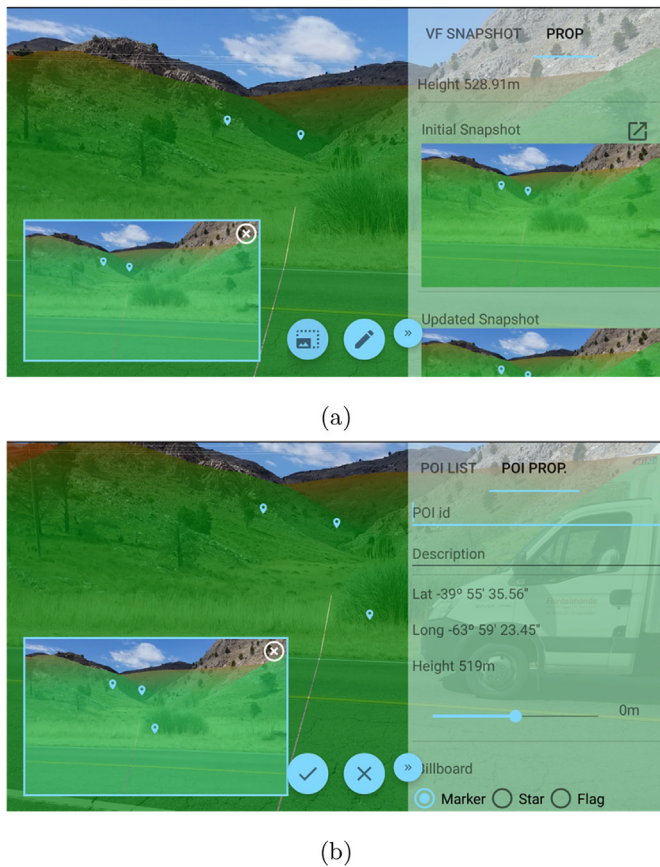
Fig. 5. The Virtual Field Snapshots are presented on the lower left corner of the screen. (a) Shows the initial Virtual Field Snapshot containing two POIs. (b) Adding a new POIs to the virtual terrain is automatically reflected on the current Virtual Field Snapshot.
