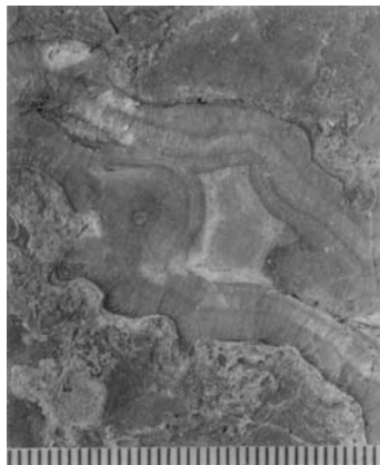
Figure 3.9 Fibrous calcite marine cement coating blocks of reef material. Note the growth layering within the cement. The central part of the cavity is filled with calcite spar. Millimetre scale. Triassic, Austrian Alps.
