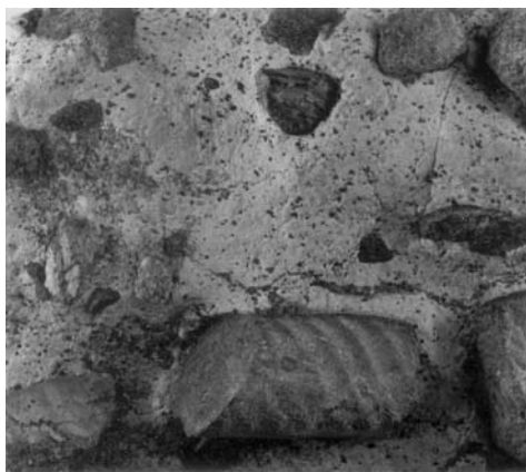
Figure 3.22 Phosphate bed composed of phosphate nodules and phosphatised fossils. The dark specks in the lime mudstone sediment are grains of glauconite (actually dark green). Specimen 10 cm across. Mid-Cretaceous, French Alps.
