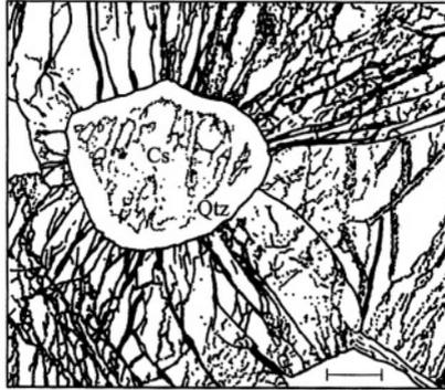
*FIG. 122*—Polymorphic transformation coesite  $\Rightarrow$  quartz in the polymetamorphic unit of the Dora Maira Massif (from a photograph in Chopin *et al.*, 1984). The coesite (Cs) which survives in inclusions in garnet is partly transformed into quartz (Qtz). The positive change in molar volume which results from this transformation bursts the garnet host creating a network of radial fractures around the inclusion. Scale is 100  $\mu\text{m}$ .
