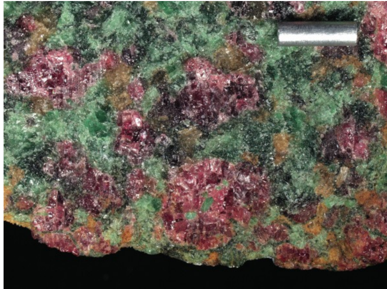
5.5 Hand-specimen of protogranular garnet lherzolite xenolith from a kimberlite (locality unknown). Chrome diopside as in Plate 5.4; yellow mineral is enstatite; garnet is red; olivine is paler green (metal rod 1 cm long). Sample courtesy of M.A. Menzies, University of London. Photo K. d'Souza.
