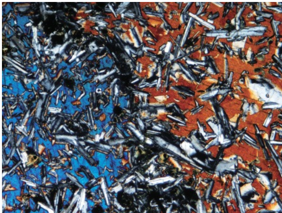
4.1 Ophitic texture in basalt (crossed polars): euhedral multiply twinned plagioclase laths (grey interference colours) are enclosed by two augite oikocrysts with first-order orange and second-order blue interference colours. Width of field 1.3 mm. (Loch Scridain, Isle of Mull.)
