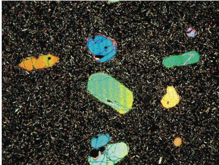
2.1 Olivine-phyric basalt from Waikoloa, island of Hawai'i (image courtesy of J.G. Fitton); Width of field 3.5 mm.
