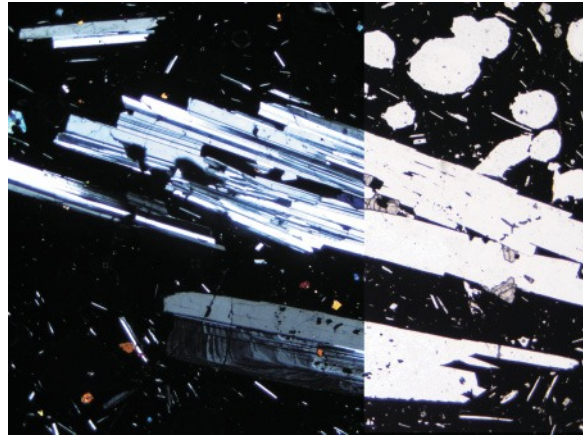
9.11 Hawaiiite lava, Canary Islands. Note oscillatory zoning in lower plagioclase phenocryst. Circular features in PPL are vesicles. Crossed polars (left), PPL (right); width of field 5.2 mm.
