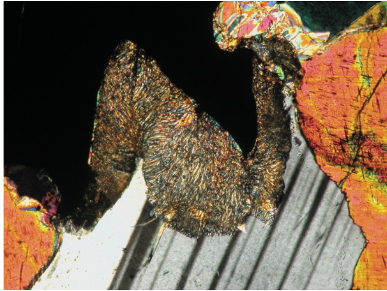
4.11 Olivine-plagioclase symplectite growing outward from the margin of a cumulus Fe-Ti oxide grain into the neighbouring cumulus plagioclase grain. Skærgaard Intrusion Middle Zone (photo courtesy of Gemma Stripp, University of Cambridge). Crossed polars, field of view 0.7 mm wide.
