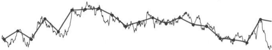
Fig. 1.2. Part of the actual trajectory and its estimate from linear regression. In this particular example, the estimated trajectory is piecewise linear because the linear regression has been carried out using an exponential covariance function
