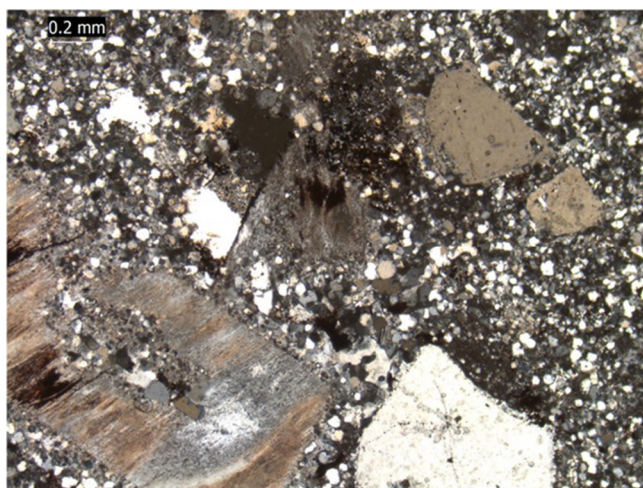
Fig. 8. Petrographic image of fresh BQP showing perthite phenocrysts in a fine grained quartz and feldspar matrix. XPL.
