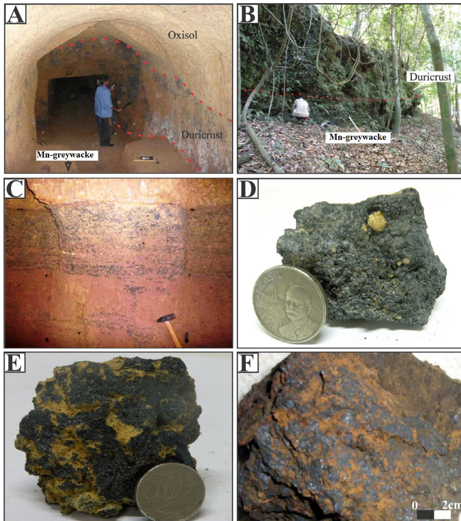
Fig. 6. Macroscopic features of the manganese deposits. (A) Galery mine of Beneficente showing Mn-greywacke, duricrust and oxisol. (B) Holanda outcrop showing the lateral extension of Mn-greywacke and duricrust. (C and D) Mn-greywackes of Holanda (A1) and Beneficente (A2), respectively. (E) Vermiform duricrust overlying the Mn greywacke of Beneficente (B1–B4). (F) Vermiform duricrust (H1–H4) overlying the Mn greywacke of Holanda.
