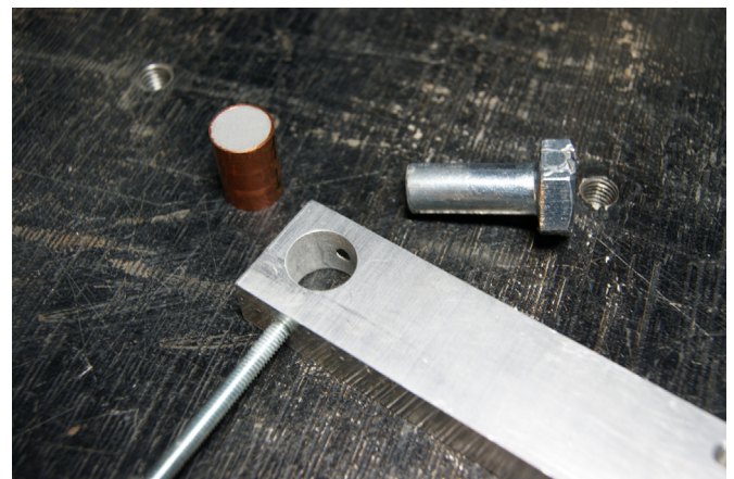
Fig. 4. Pulverised sample made into a pellet (on the left) and tools used to produce one (see also Kauppinen et al. (2014a)).
