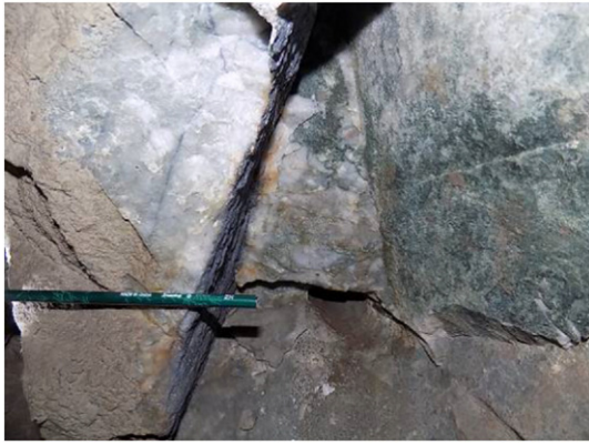
Fig. 13. Molybdenum hosted in structural fracture in quartz sandstone (Lindi formation).
