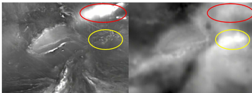
Fig. 14. Images of the Sudbury Structure offset to the left of centre for each, and the Temagami anomaly in the top right corners. The left image is of the magnetic data and the right image is of the gravity data. The red ellipse highlights the mentioned magnetic anomaly, which is clearly is the largest highly magnetic portion of the map. The yellow ellipse shows an area with low magnetic values but a higher gravity anomaly. (For interpretation of the references to color in this figure legend, the reader is referred to the web version of this article.)
