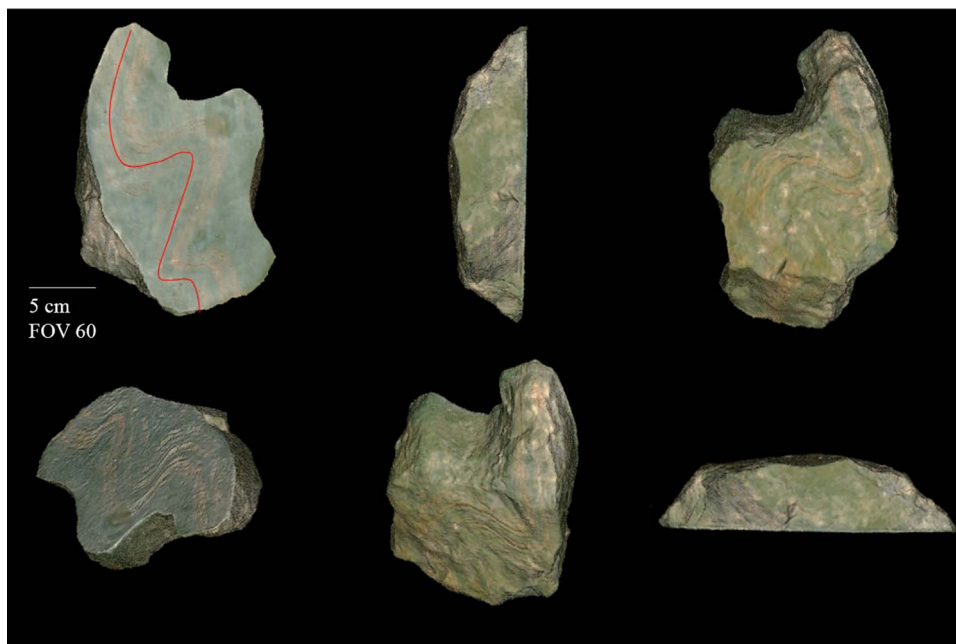
Fig. 10. Paragneiss sample from the Perth Road mylonitic outcrop. Note the intense anastomosing fold bands within the sample, highlighted in the first view in red. Scale information is shown for the first depiction.
