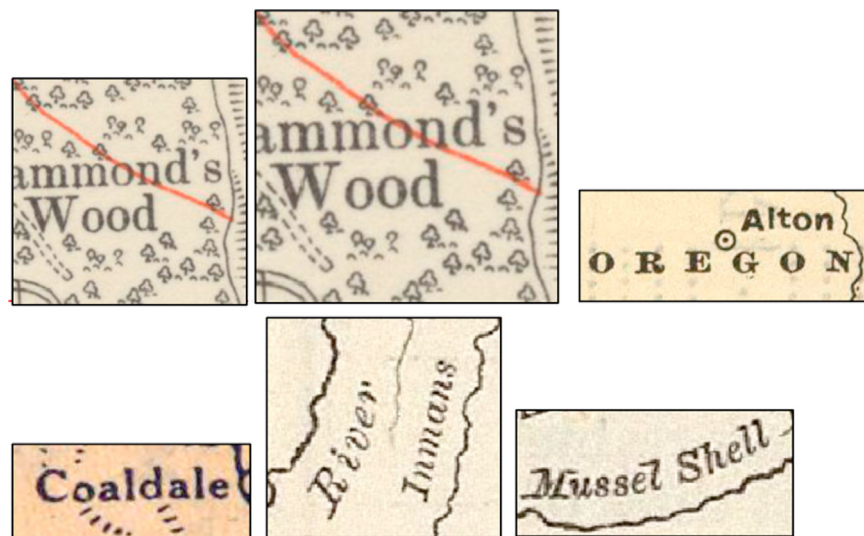
Fig. 20. Example labels that are in noisy areas where nearby non-text symbols (e.g., trees, terrain features, circular symbols) could mislead the text detection and recognition algorithms (top), are slightly distorted or moderately curved (bottom) (Group 2).
