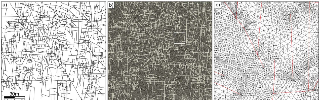
Fig. 9. Converting a deterministic fracture network into a triangular mesh: a) 150 m×142 m section extracted from an outcropping carbonate pavement in the Potiguar basin (NE Brazil); b) Meshed fracture network geometry; c) detail of the mesh showing refinement around the fracture terminations and intersections (location indicated by the white square in (b)).
