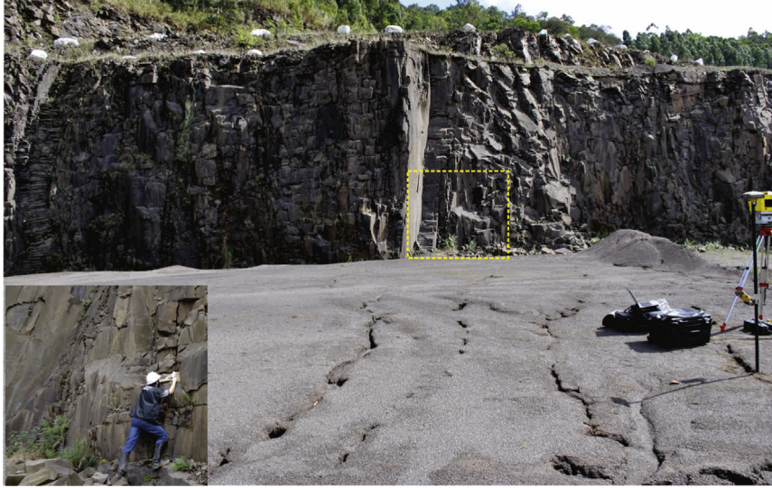
Fig. 1. Global view of the basalt quarry where the dataset was acquired using a laser scanner (visible at the right-hand side of the photograph). The whole outcrop is about 10 m high and 40 m long. The inset shows the three main fracture families and in situ manual orientation using a compass and clinometer. (For interpretation of the references to color in this figure caption, the reader is referred to the web version of this paper.)
