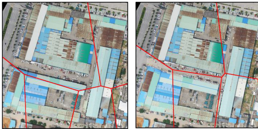
Fig. 5. A large ground structure in the image. Red lines are initial seam-line network; the vertices (conjunction node) in the image to the left are mostly located on the buildings while the vertices in the image to the right have been moved to near the ground. (For interpretation of the references to colour in this figure legend, the reader is referred to the web version of this article.)
