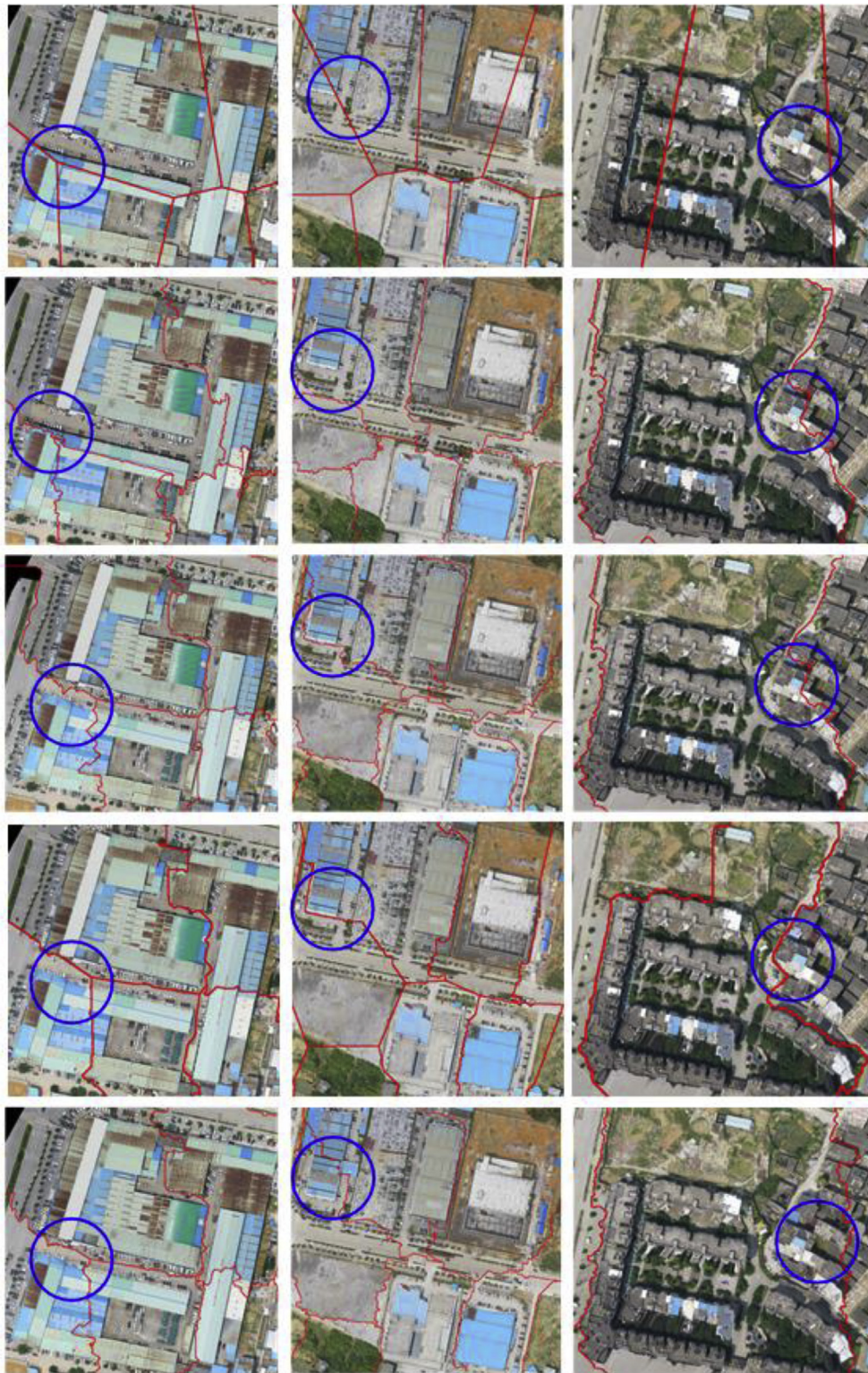
Fig. 9. Comparison of initial seam-lines and the optimized seam-lines with the dataset 1 in details. The five rows of images from top to bottom show the initial seam-lines, the seam-lines refined by Chon's method, VR-Chon's method, the proposed method, and the DSM-Color method respectively. The blue circles mark the main differences of different methods. (For interpretation of the references to colour in this figure legend, the reader is referred to the web version of this article.)
