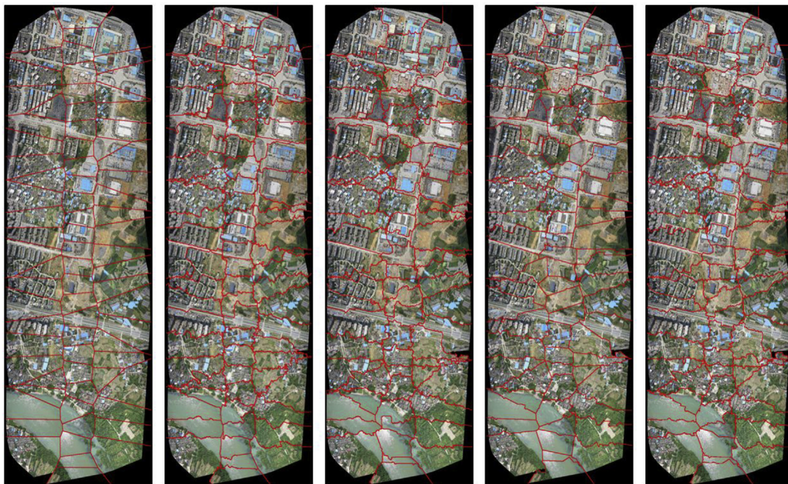
Fig. 8. Comparison of the initial and refined seam-line networks on dataset 1. The images from left to right are the initial seam-line network, the seam-line network refined by Chon's method, VR-Chon's method, the proposed method, and the DSM-Color method respectively. The red lines in the images are seam-lines. (For interpretation of the references to colour in this figure legend, the reader is referred to the web version of this article.)
