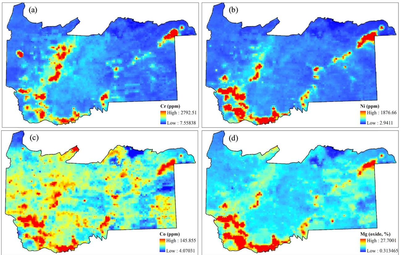
Fig. 4. Spatial distribution of four geochemical elements mapped by IDW interpolation (a) Cr, (b) Ni, (c) Co, and (d) Mg.
