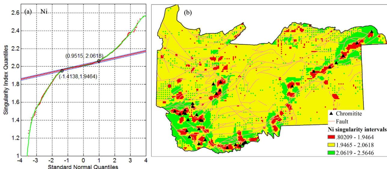
Fig. 8. (a) Ni singularity index quantiles vs. standard normal quantiles, and (b) singularity map with categorical values based on S-Q analysis. (For interpretation of the references to color in this figure legend, the reader is referred to the web version of this article.)
