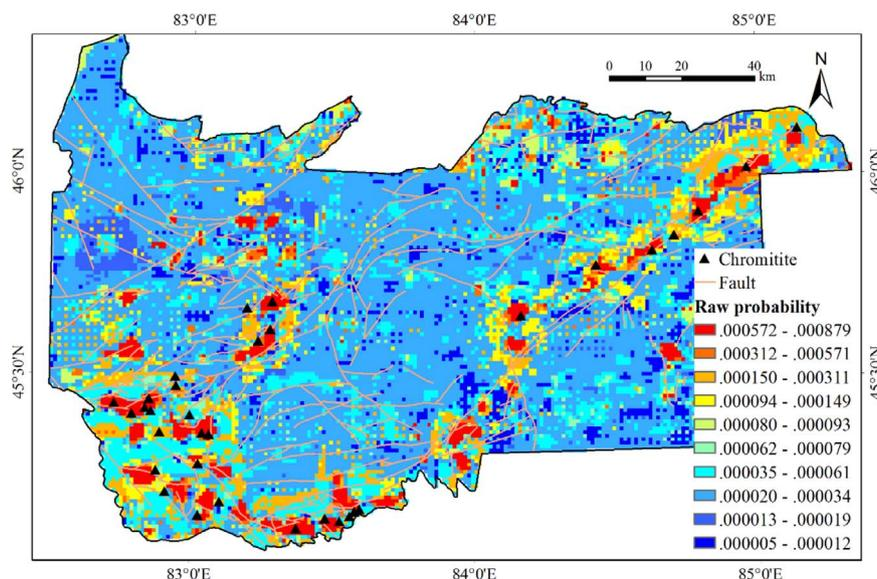
**Fig. 11.** Chromitite prospectivity map produced by optimized geochemical anomalies using MaxEnt model.
