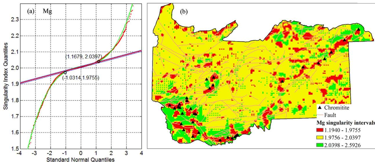
**Fig. 10.** (a) Mg singularity index quantiles vs. standard normal quantiles, and (b) singularity map with categorical values based on S-Q analysis. (For interpretation of the references to color in this figure legend, the reader is referred to the web version of this article.)
