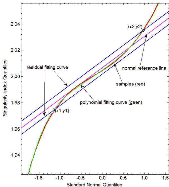
Fig. 2. Illustration of S-Q method in frequency domain.
