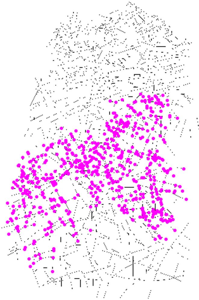
Fig. B.5. The largest connected network in sample JT-6. The labels in circles represent the nodes or intersections of fracture traces that form the main component. In picture, the traces look like discontinue lines however if we look very closely they are solid lines.
