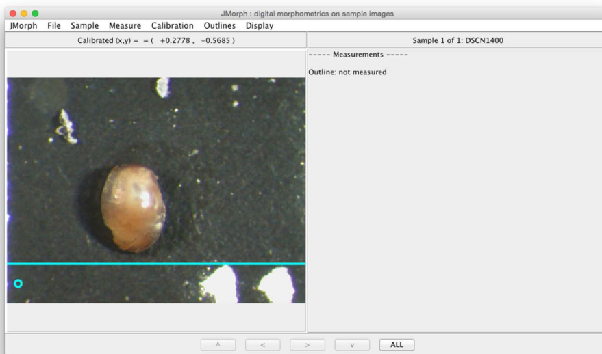
Fig. 4. The JMorph GUI with a sample image loaded and calibrated, and a single measurement defined. The calibration length is drawn as a cyan line. The calibration origin is drawn as a cyan circle.
