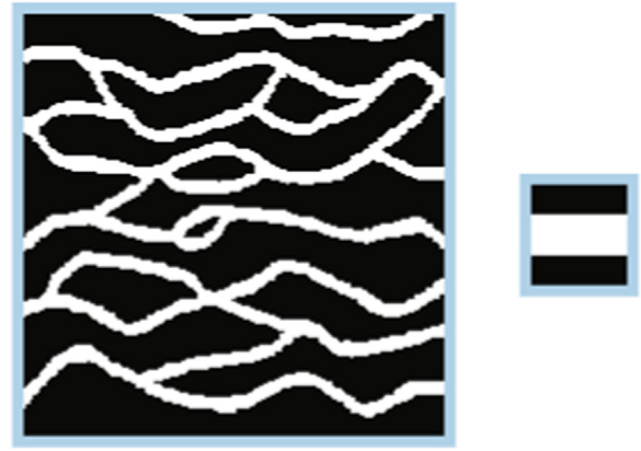
Fig. 4. Nearly all patterns of this binary channelized image (251 by 251 pixels) can be reconstructed by applying simple mappings (like rotation and translation) to the elementary pattern depicted besides the image. Therefore the space of the patterns in this image has very low effective dimensionality.
