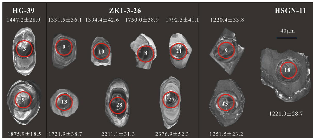
Fig. 5. CL images of zircon grains in metasedimentary rocks (HG-39 and ZK1-3-26) and diabase sample (HSGN-11). The circles are analysis spots marked with ages (Ma).
